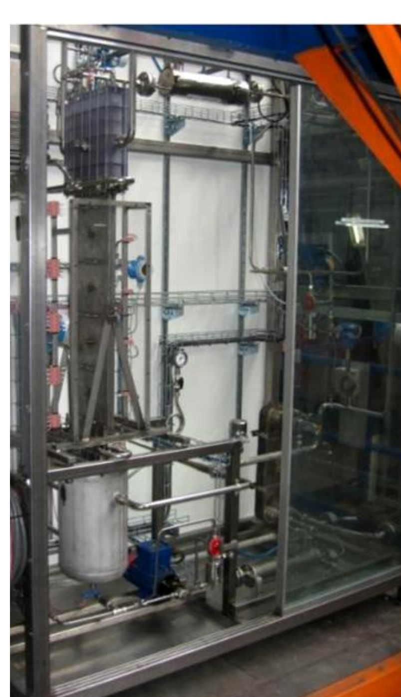
Figure 2: HIDiC (left) before insulation, flow sheet (right) showing sampling points
