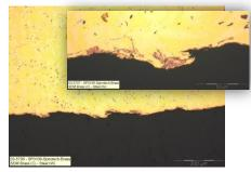
SDM test: Brass vs C-steel Results: 10hrs
