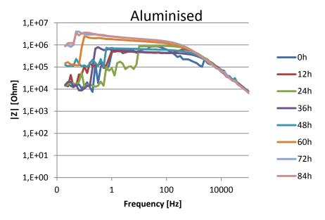
Low resistance → High electrochemically active → corrosion
