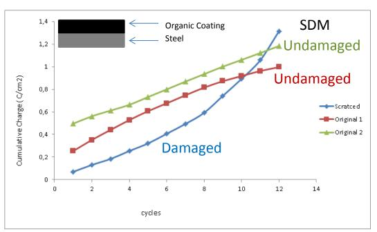
Undamaged: straight climbing line → electrochemical stable behaviour → relative protective layer
