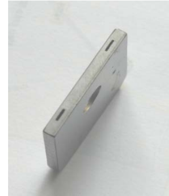
Internal voids e.g. cooling channels possible
