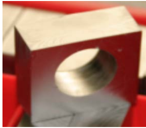
As sintered mono-blocks and mock up for ITER divertor target
