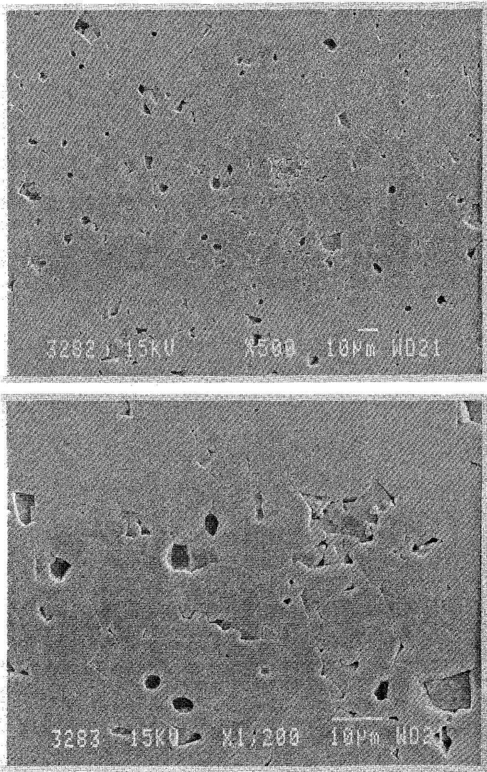
Figure 2.1. The microstructure of Wesgo Al 995.
