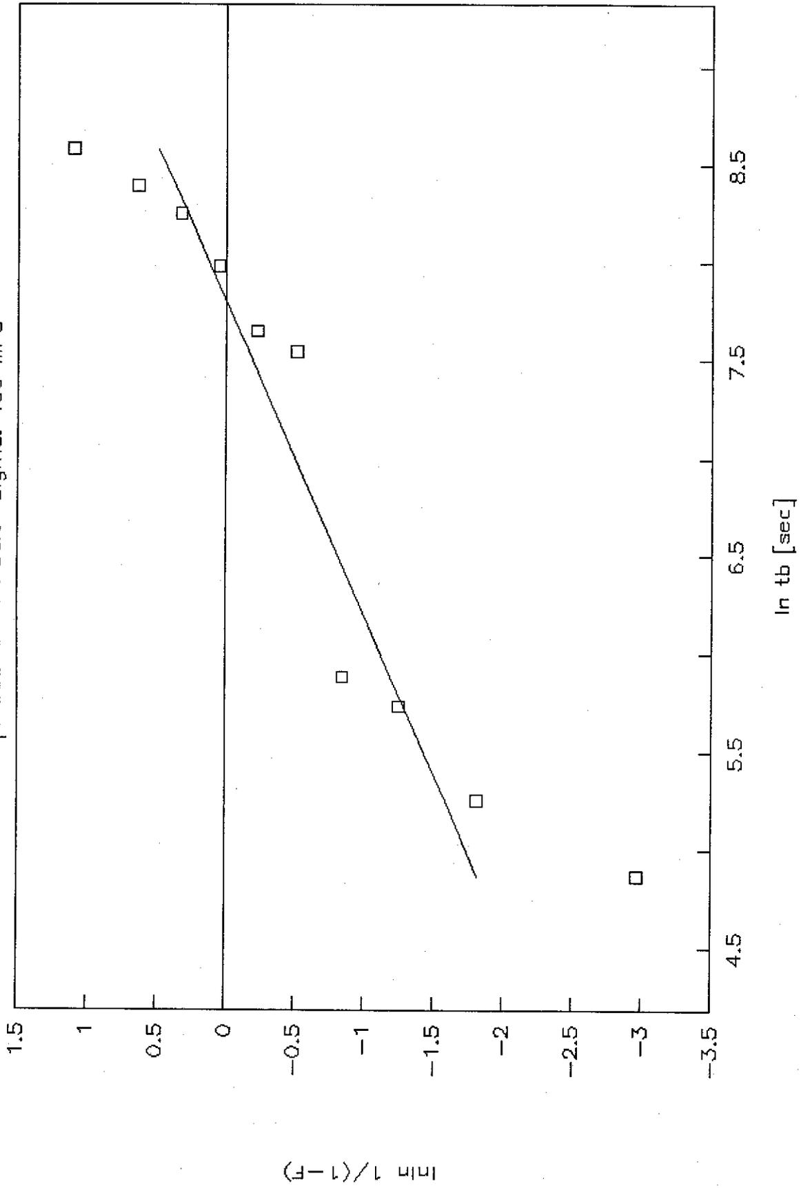
Fig. 3.2. Weibull plot of the time-to-fracture data for  $\sigma = 100$  MPa.
