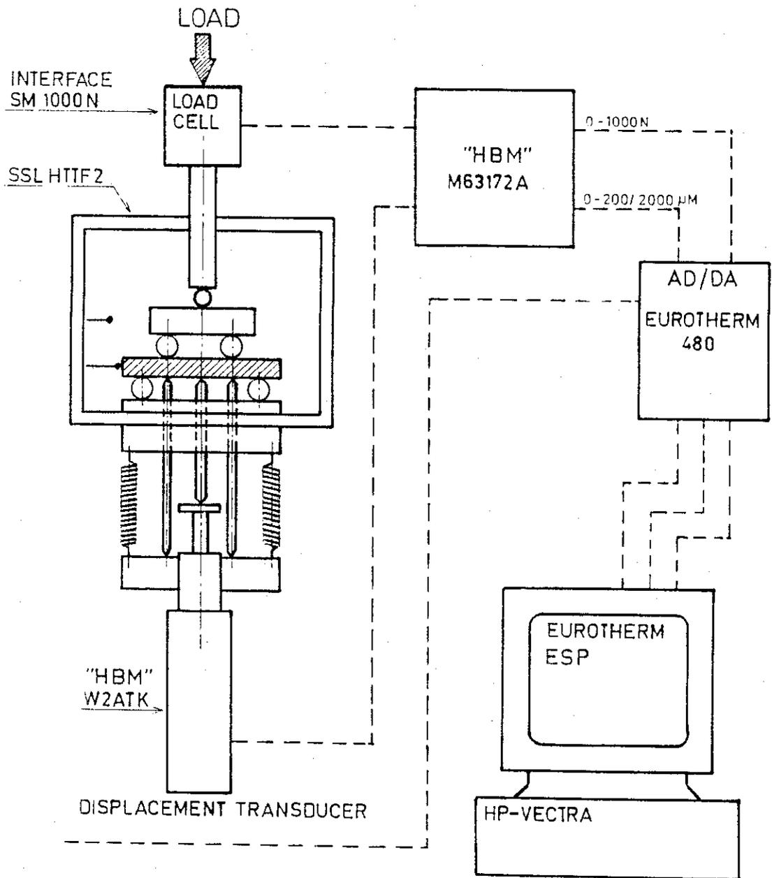
Fig. 2.2. Experimental set-up for the time-to-fracture tests.
