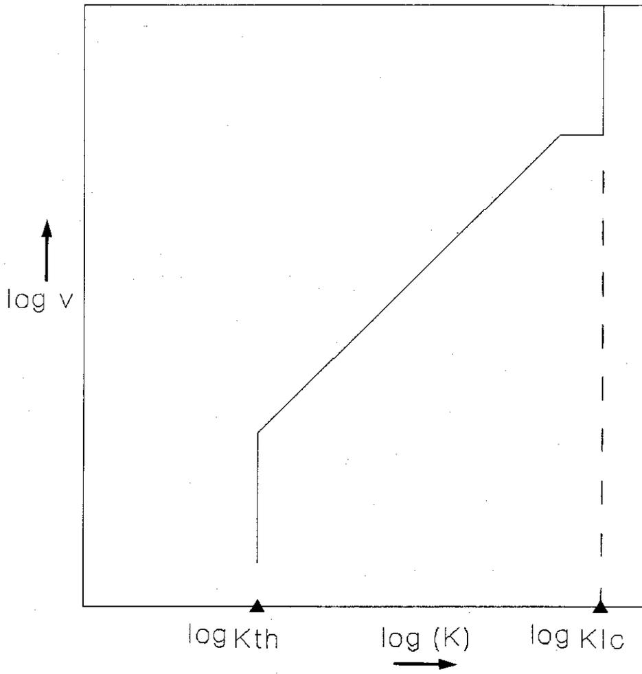
Fig. 1.1. Typical subcritical crack growth curve.
