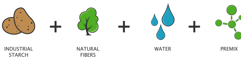
Figuur 4 The PaperFoam recipe consist of starch, fibers, water and a premix
