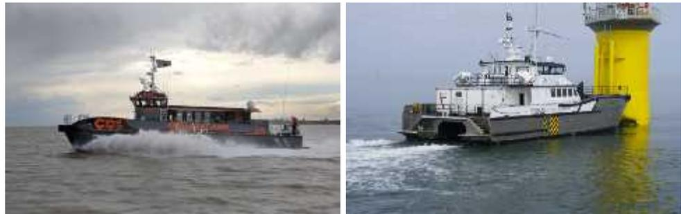
These workboats not only have higher capacity and workability, but also have higher speeds of travelling. Since the travelling time is also counted as the working time [9], for far-offshore wind farms, the actual working window on wind turbine is less. Such workboats facilitates safe and fast transfer of crew and small spare parts.
