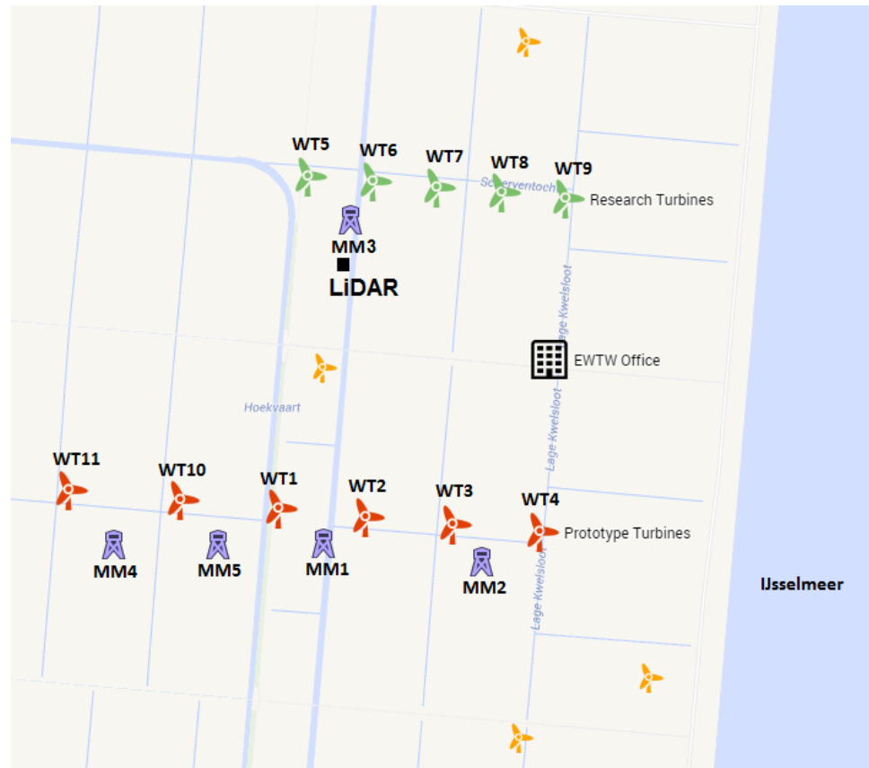
Figure 2: Layout of the test site EWTW: the meteorological mast 3 is surrounded by 5 research turbines (WT5 – WT9), 6 prototype wind turbines (WT1 –WT 4,WT 10,WT 11) and 4 smaller single wind turbines. The location of the ground based LiDAR is denoted by the black square south of the meteorological mast 3.
