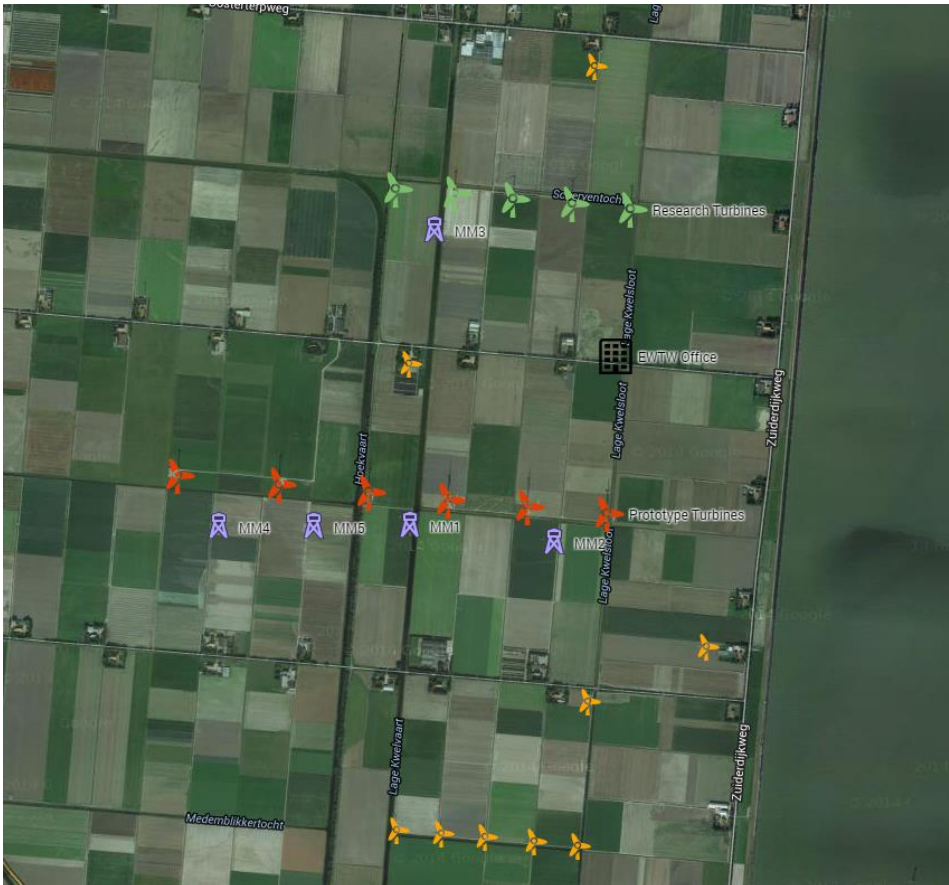
Figure 7: The EWTW infrastructure from satellite view: research turbines in green, prototype locations in red, neighbour turbines in orange and meteorological masts in purple [Google]
