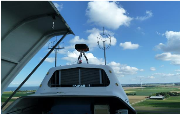
Figure 19: Wind Iris at the back of the nacelle of Nordex 6
