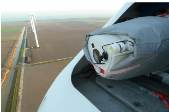
Figure 20: photograph of the Zephir located on the back of the nacelle of Nordex 6
