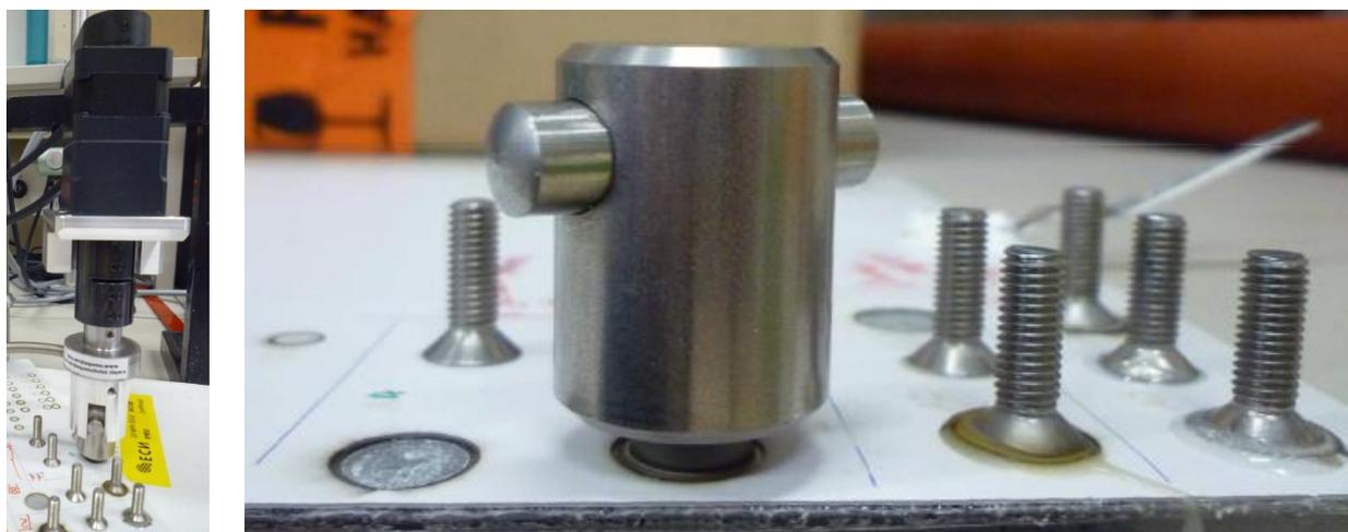
Figure 4.1: Left: overview image of the core/shear set-up. Right: detail of the torque-head.
