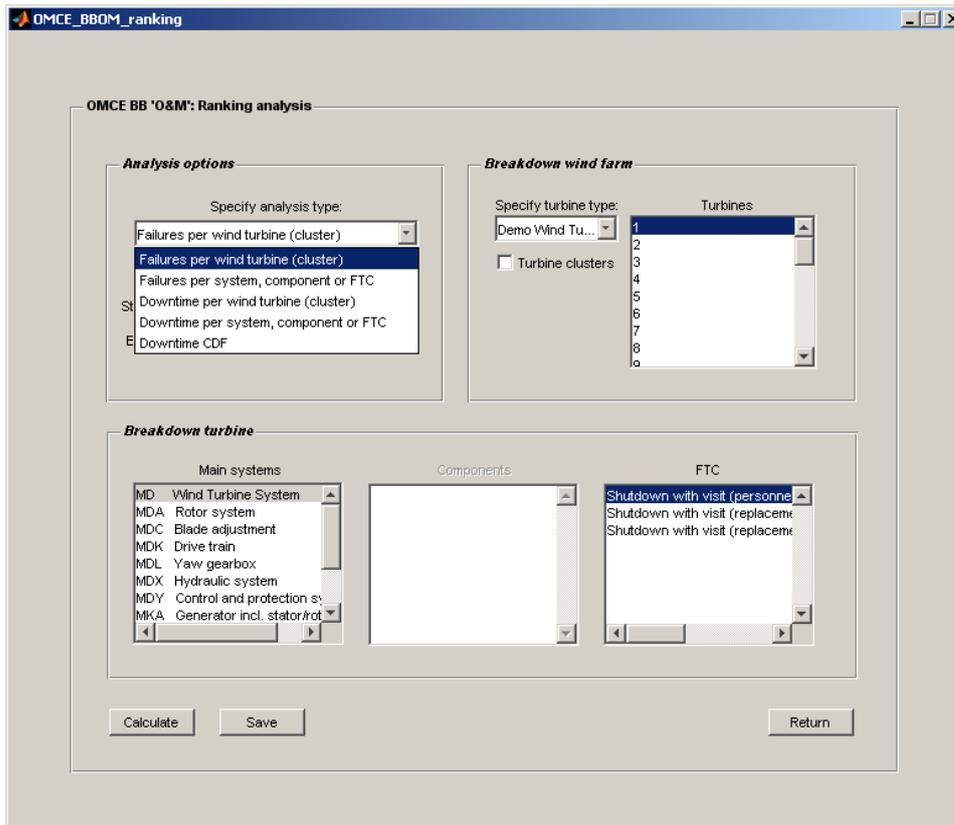
Figure 12-8 The ranking analysis menu of the OMCE Building Block 'Operation & Maintenance'.
