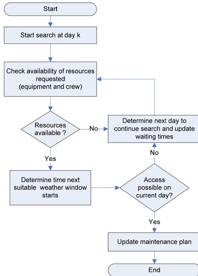
Figure 6-4: *Process flow of insertion of replacement*
