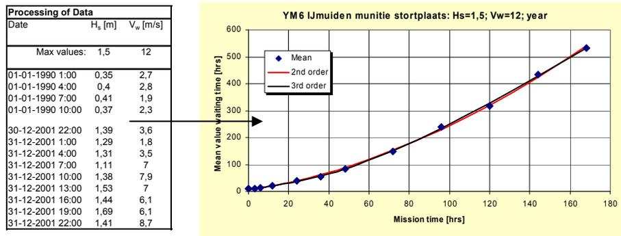
Figure A-3: *Example of determining relationship between average waiting time and mission time*
