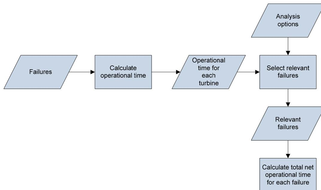
Figure 12-4 *Pre-processing process for analysis of maintenance data.*
