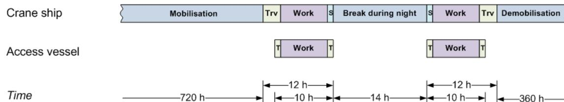
Figure 8-12: Breakdown of repair mission for defined replacement with 16 hours of work performed by 2 vessels
