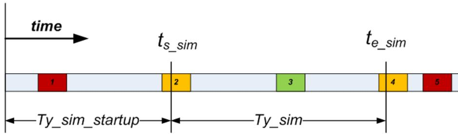
Figure 7-1: *Simulation period and possible repairs due to simulation period selection;  $t_{s\_sim}$  and  $t_{e\_sim}$  are the start time and the end time of a certain simulation period (i.e. the next 1, 2, ..., 5 years), and  $Ty\_sim\_startup$  is the start-up period*
