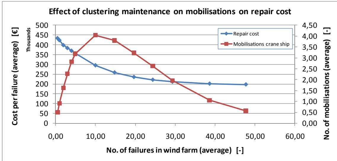
Figure 8-13: Effect of clustering maintenance on number mobilisations and repair cost
