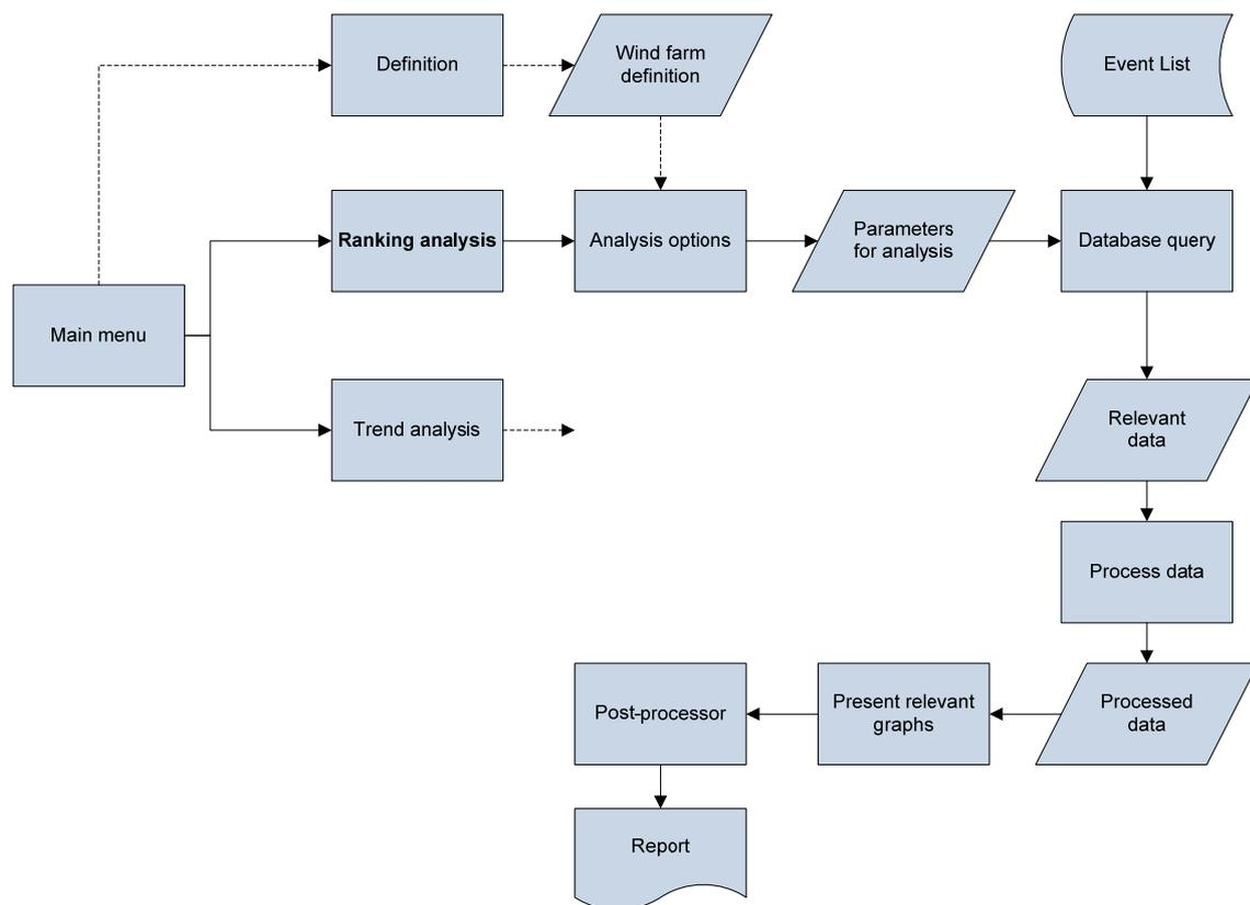
Figure 12-1 *Flowchart for performing ranking analysis of the maintenance data using the building block 'Operation & Maintenance'.*
