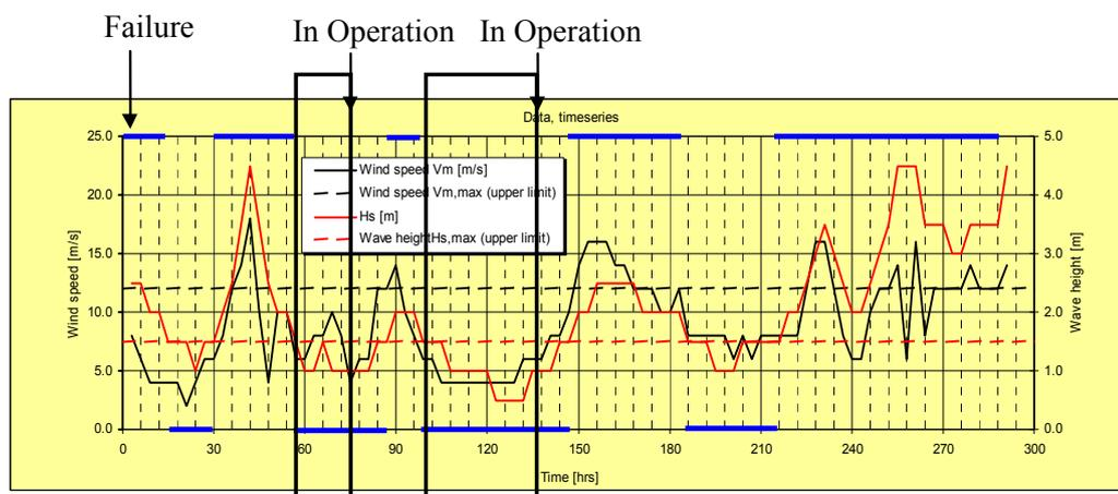
Figure B.4: *Example of determination of waiting time for a maintenance action that can be carried out if  $H_s \leq 1.5$  m and  $V_w \leq 12$  m/s and the duration is 20 hrs or 40 hrs.*
