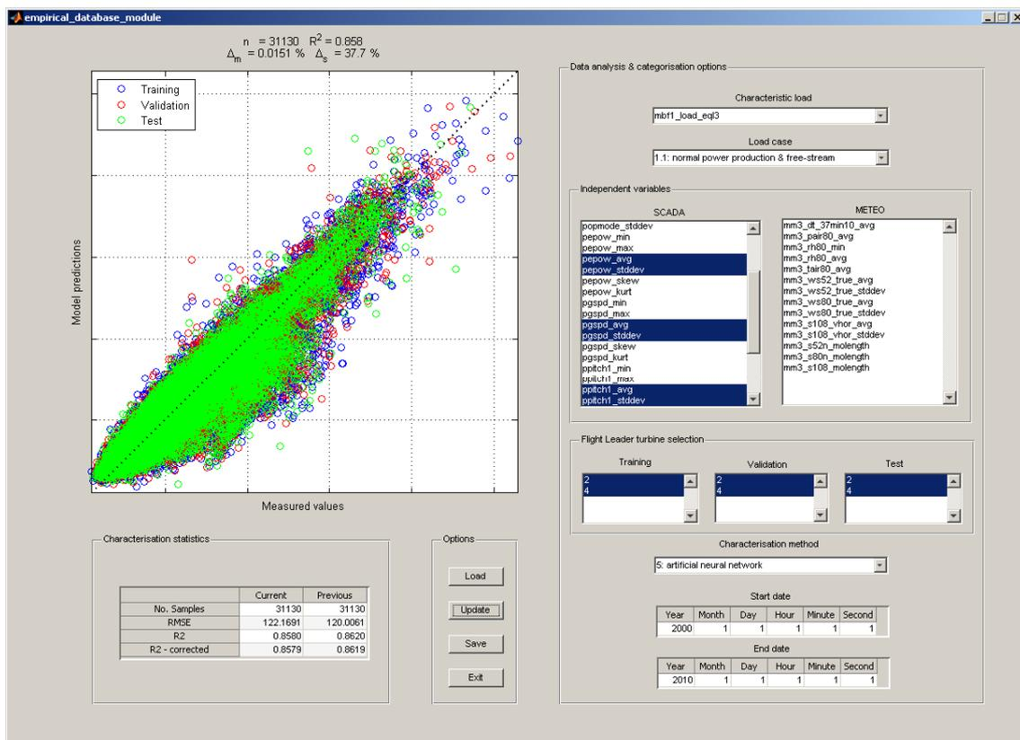
Figure 14-4 The Flight Leader's empirical database module for establishing relations between SCADA parameters and load indicators.
