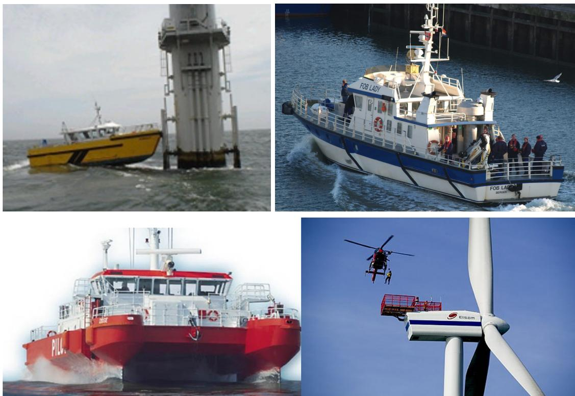
Figure 2-4: Examples of transportation and access equipment for maintenance technicians; clockwise: Windcat workboat, Fob Lady, helicopter, and SWATH boat
