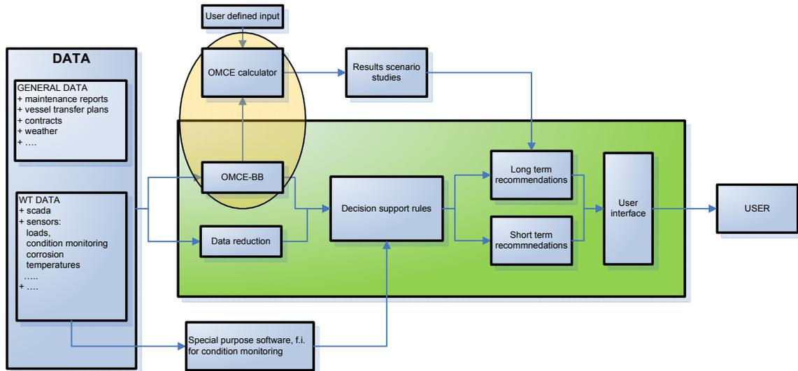
Figure 3-2: Structure of the D OWES system for optimising O&M of offshore wind farms in the long and short term making use of wind farm data. The green rectangle represents the portal from which all data sources and models can be approached. The orange oval represents the OMCE concept. The OMCE-Calculator uses the data processed by the OMCE BB's as input.
