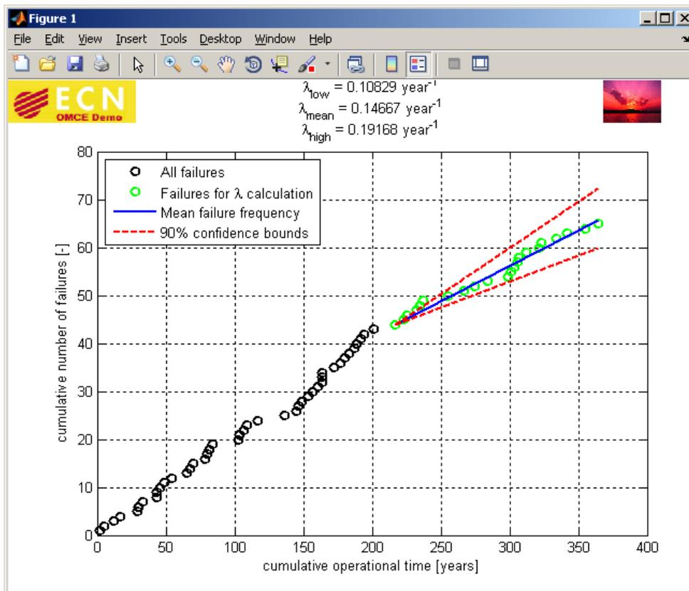
Figure 12-11 Example of the output of the trend analysis of OMCE Building Block 'Operation & Maintenance'.
