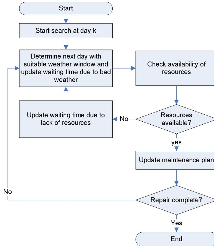
Figure 6-6: *Process flow of insertion of inspection or repair*
