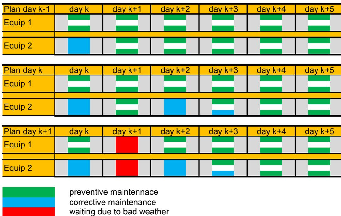
Figure 6-1: Schematic overview for development of an integral maintenance plan
