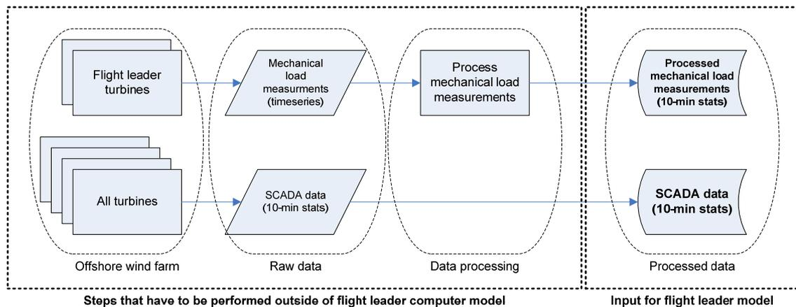
Figure 14-3 *Flowchart indicating the different steps for generating the (measured) input (SCADA and mechanical load measurements) data for the Flight Leader computer model.*
