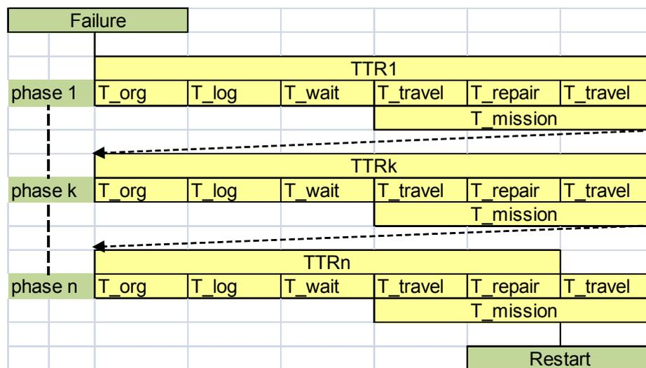
Figure 5-3: Sequence of maintenance phases
