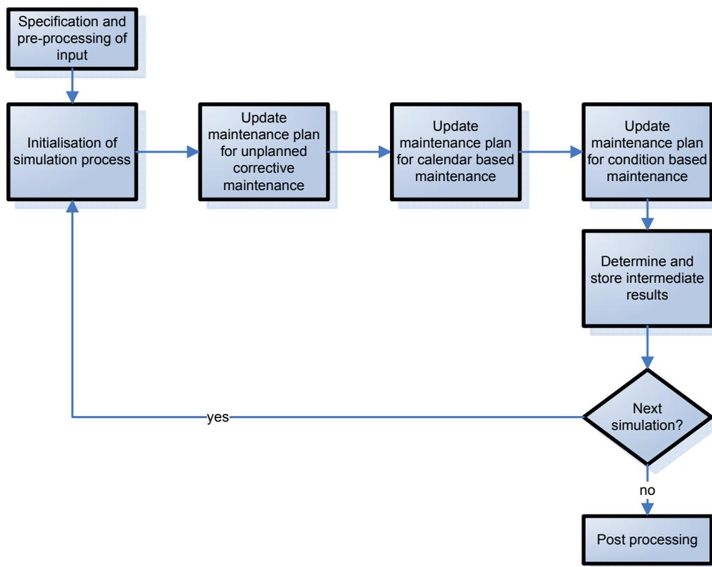
Figure 6-2: *Basic schematic overview of the modelling process of the different types of maintenance.*
