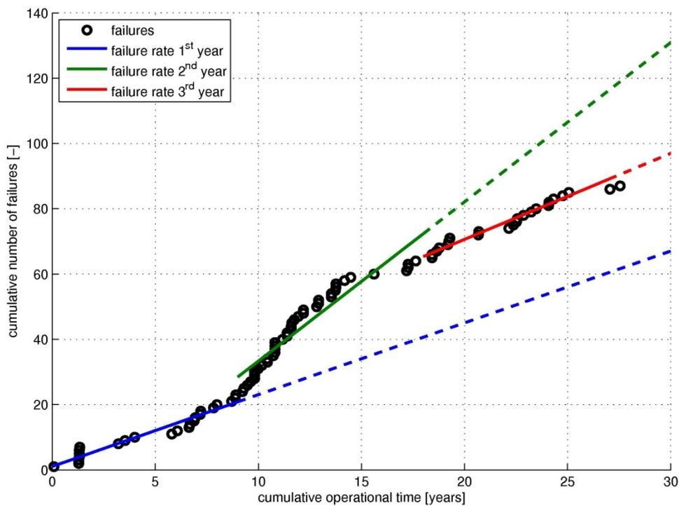
Figure 12-5 Example of a CUSUM-plot used for visualizing trends in failure behaviour.
