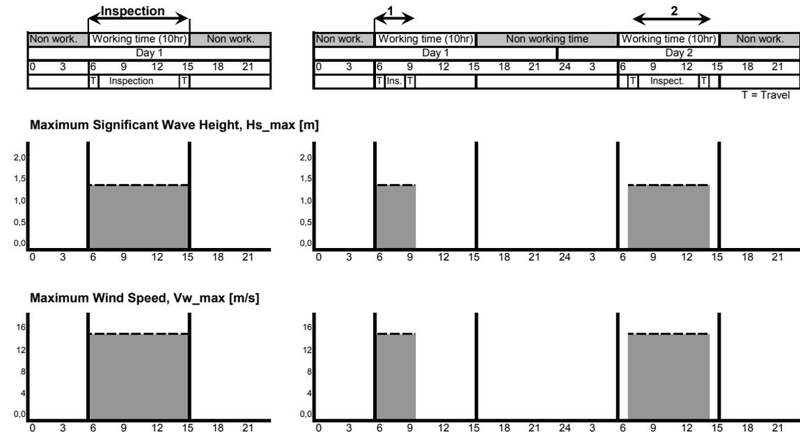
Figure 5-5: "Inspection" of 8 hrs with 1 hour travelling to and from the turbine
