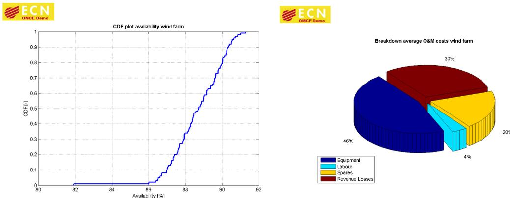
Figure 8-8: OMCE-Calculator post-processor plot output, CDF availability wind farm (left) and breakdown of O&M costs wind farm (right)
