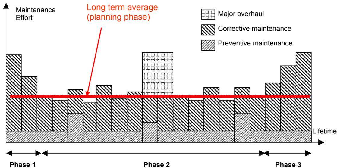
Figure 2-8: *Schematic overview of the maintenance effort over the lifetime of a turbine. In reality, none of the lines is constant; the actual maintenance effort will vary from year to year.*
