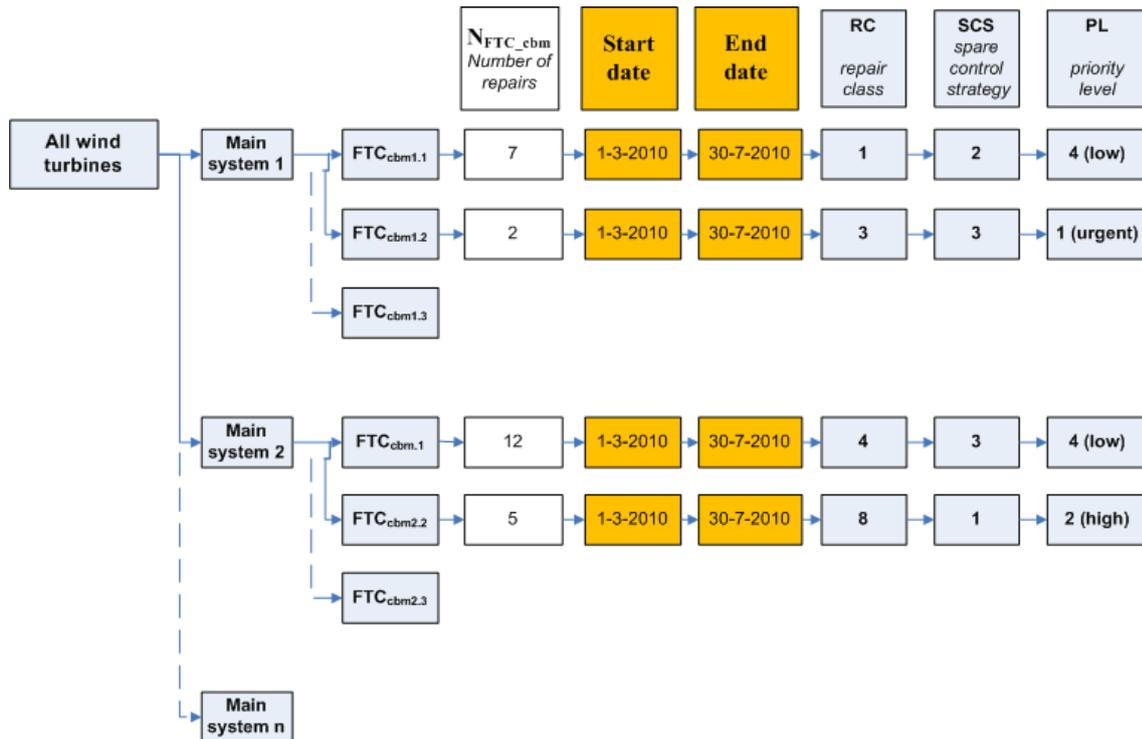
Figure 5-8: Definition of FTC's for condition based maintenance (subscript "cbm" = condition based maintenance)
