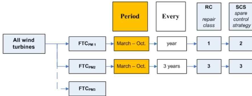
Figure 5-9: *Definition of FTC's for calendar based maintenance (subscript "pm" = preventive maintenance)*
