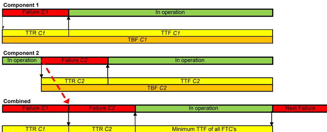
Figure B.3: Illustration of two component failures and the delay in repair of component 2
