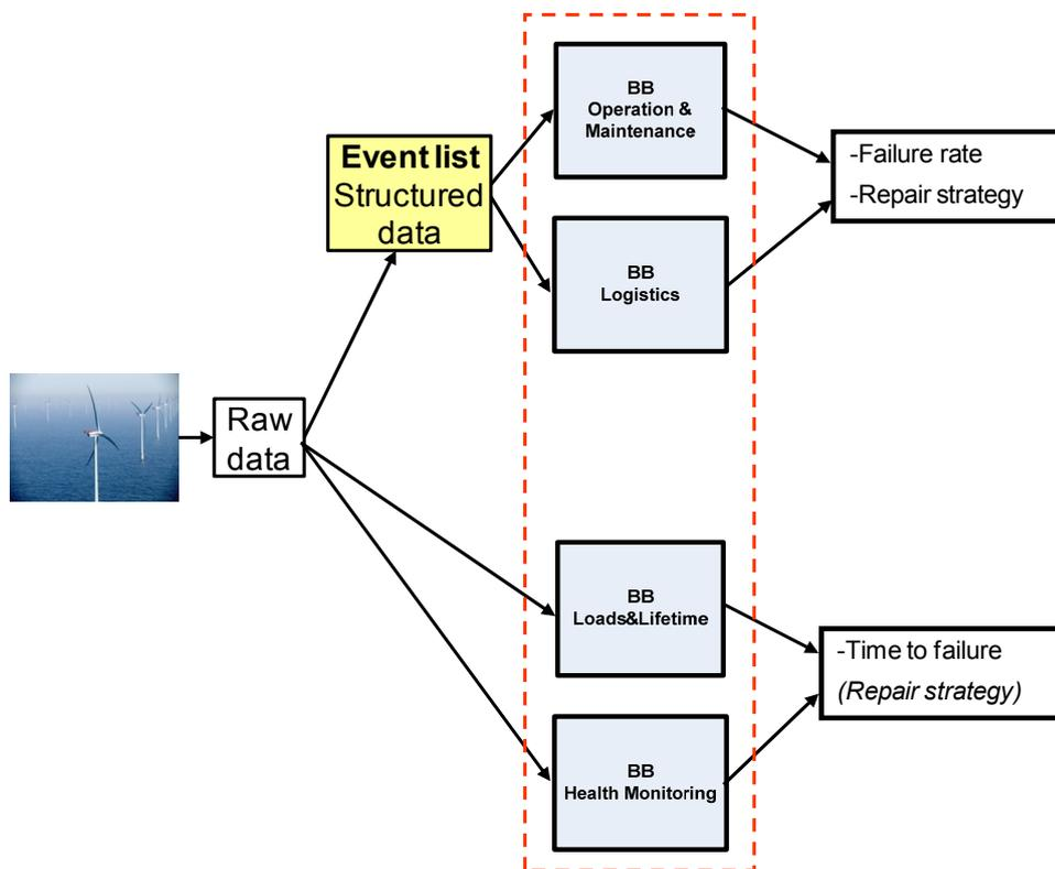
Figure 9-1: Relationship between the raw wind farm data, the Event List and the OMCE BB’s
