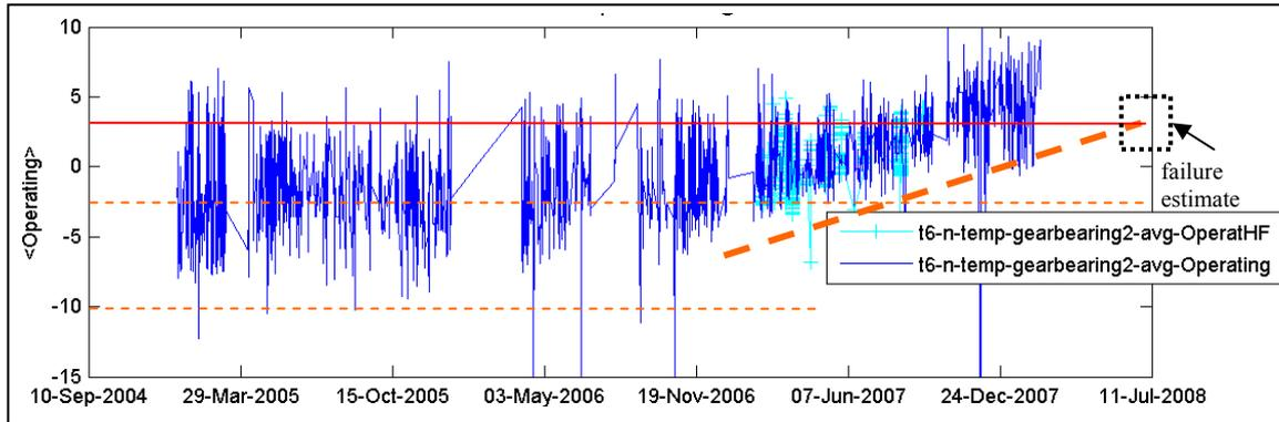
Figure 15-1: *Example of a visualisation from de-trended SCADA statistical data; slow increase of the bearing temperature indicating wear*
