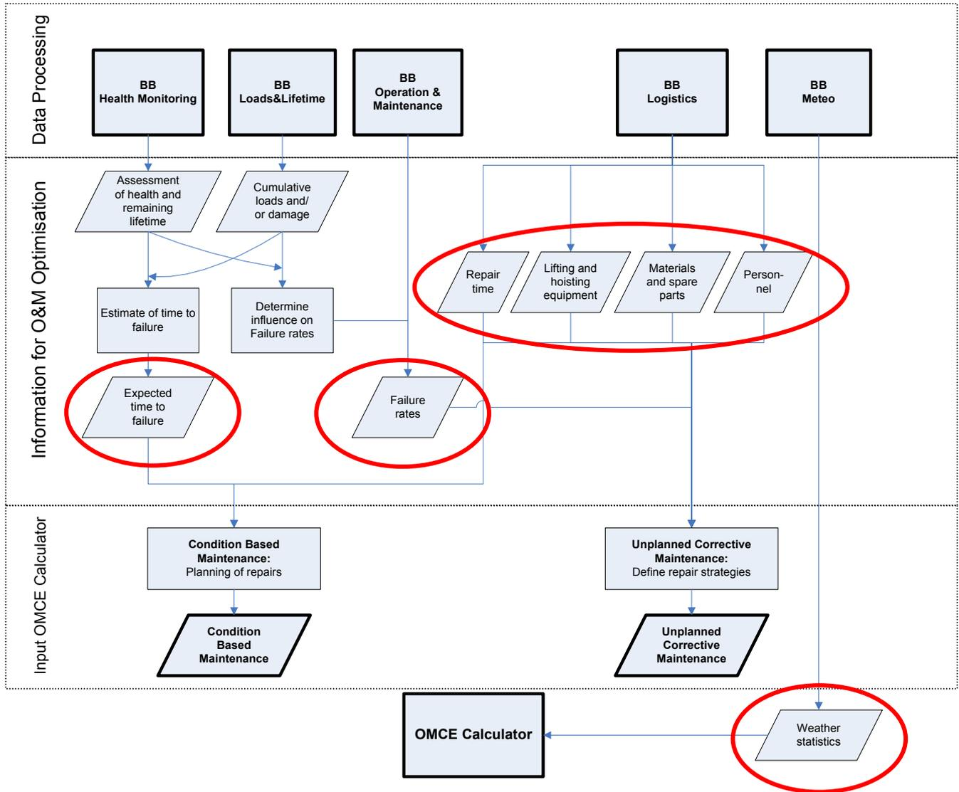
Figure 9-2: Interfaces between the OMCE-BB's and OMCE-Calculator
