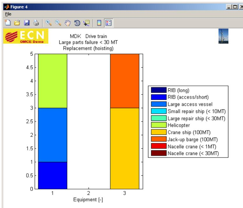
Figure 13-5 Example of the output of the Repair Class (RPC) characterisation of the Building Block 'Logistics'. Here the usage of equipment is shown for a large replacement of the drive train.
