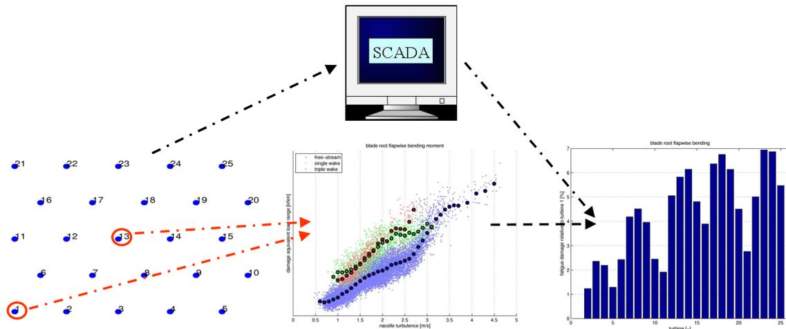
Figure 14-1 *Illustration of the Flight Leader concept; the load measurements performed on the Flight Leader turbines (indicated by the red circles) are used to establish relations between load indicators and standard SCADA parameters; these relations are combined with the SCADA data from all other turbines in the wind farm in order to estimate the accumulated loading of all turbines in the farm.*
