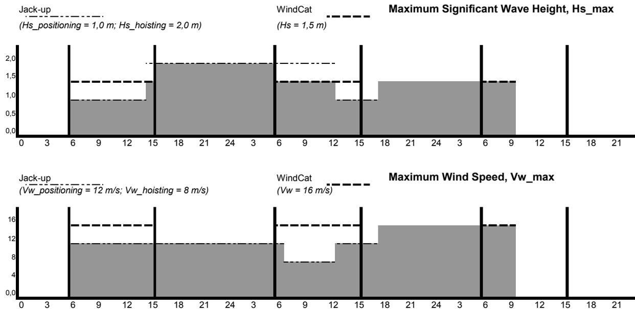
Figure 5-6: "Replacement" of gearbox; maximum allowable weather conditions indicated as grey areas
