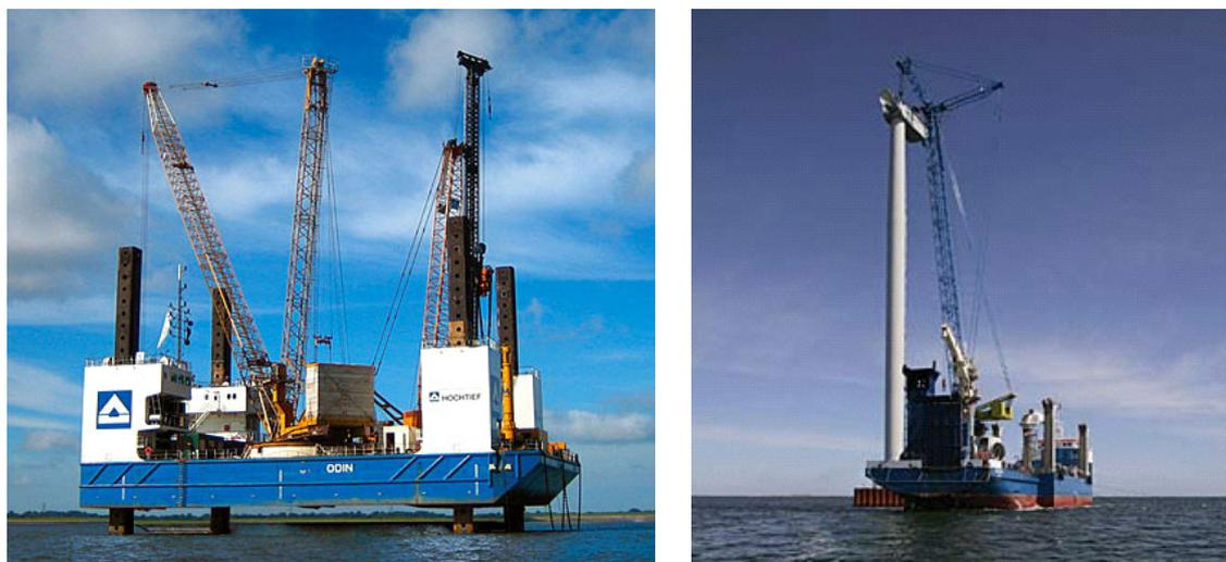
Figure 2-5: Examples of external cranes for replacement of large components; Jack-up barge ODIN (left) and crane ship Sea Energy (right)
