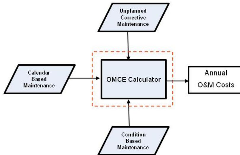
Figure 4-1: *OMCE Calculator to model 3 types of maintenance and estimate O&M aspects*
