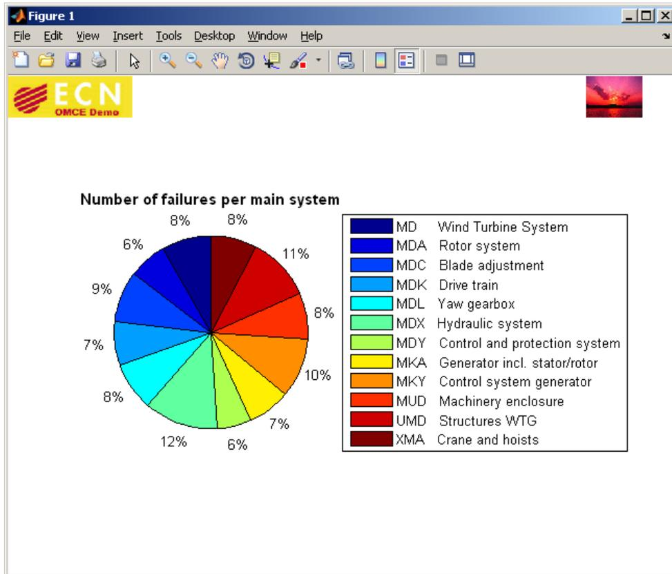
Figure 12-9 Example of the output of the ranking analysis of OMCE Building Block 'Operation & Maintenance': Number of failures per main system.
