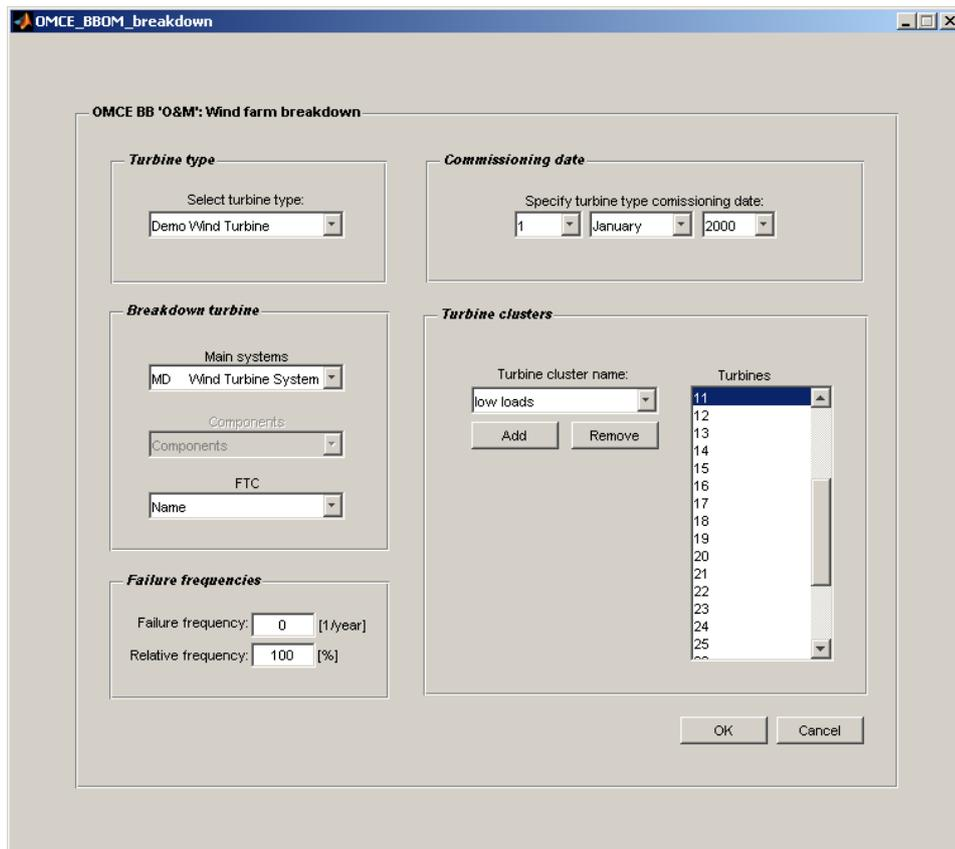
Figure 12-7 The wind farm breakdown menu in the OMCE Building Block 'Operation & Maintenance'.
