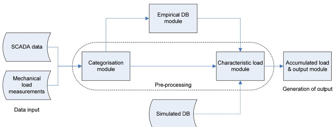
Figure 14-2 *General structure for the Flight Leader computer model.*
