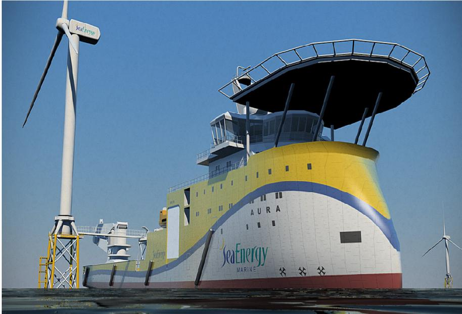
Figure 2-6: *Impression of Sea Energy's Ulstein X-bow [Ref. 26]*
