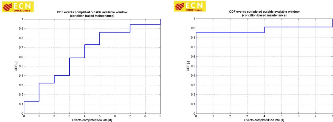
Figure 8-14: CDF plot of number of maintenance events performed outside required maintenance period; Simulations with 1 vessel available (left) and simulations with 2 vessels available (right)
