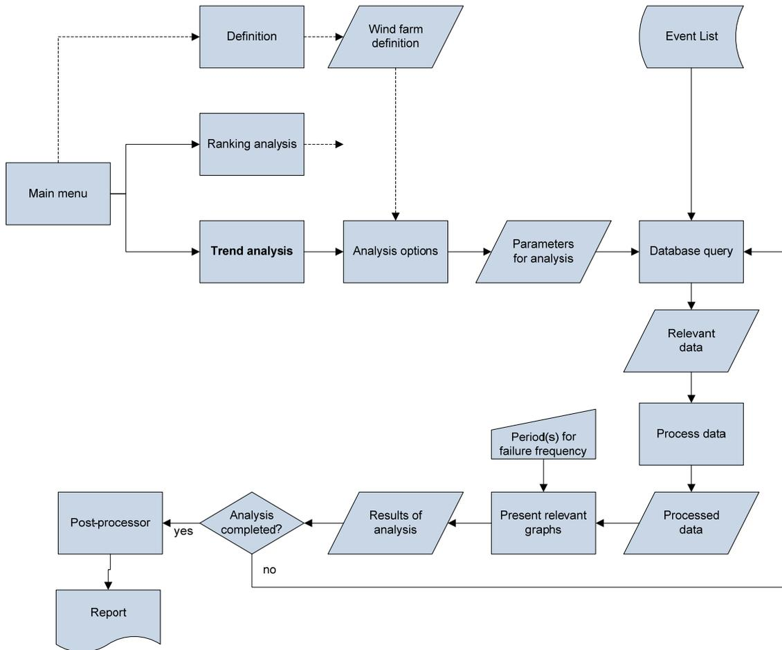
Figure 12-2 Flowchart for performing trend analysis of the maintenance data using the building block 'Operation & Maintenance'.
