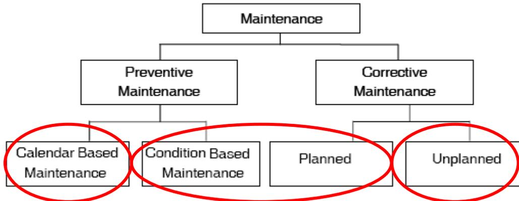
Figure 2-7: Schematic overview of the different types of maintenance [Ref. 11]
