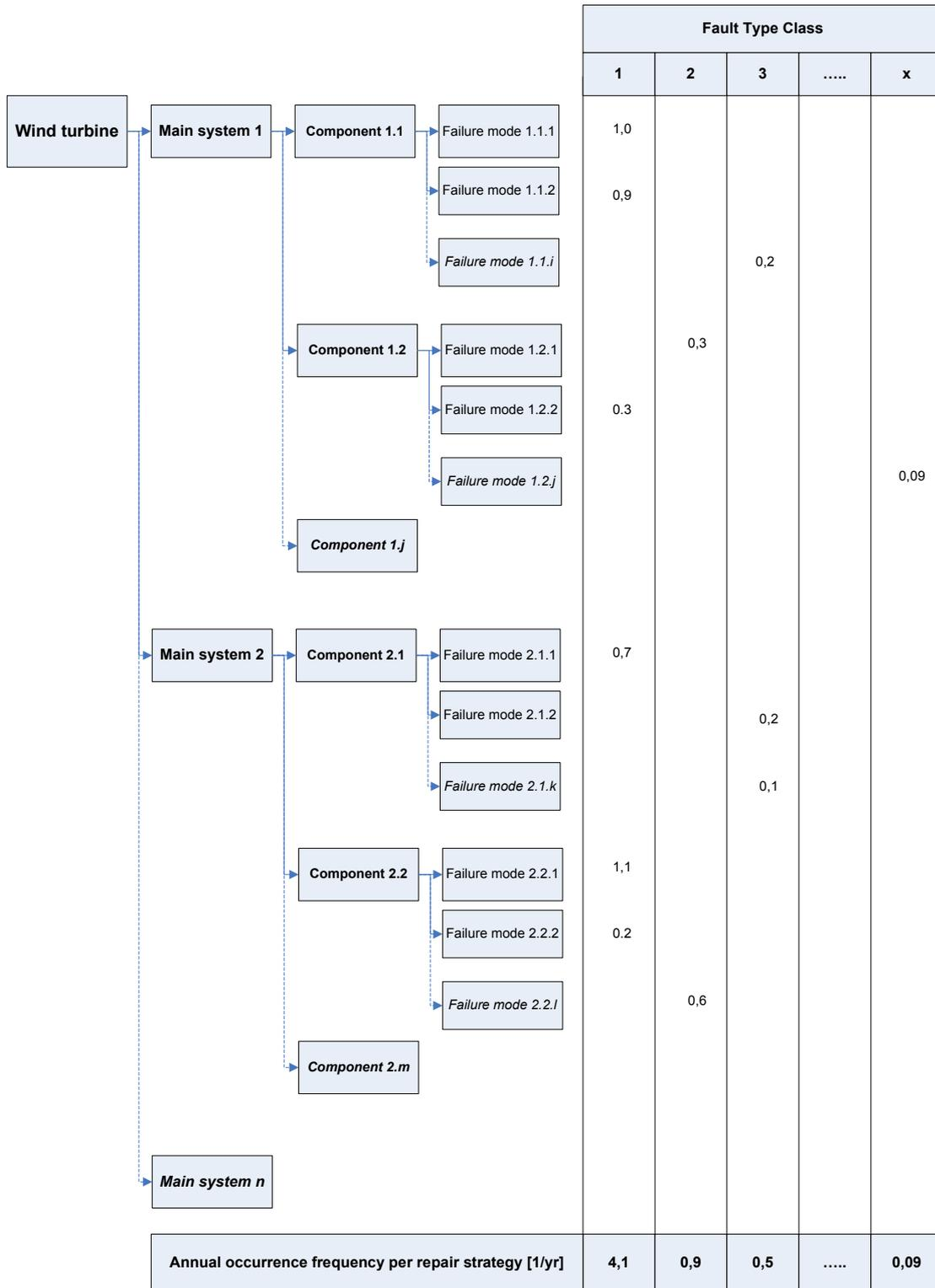
Figure 5-1: Example of grouping failure modes into manageable set of fault type classes
