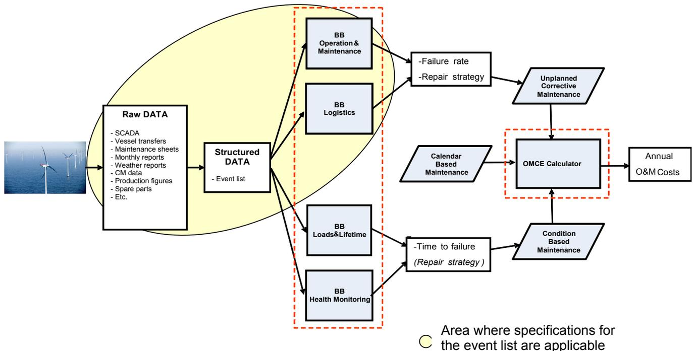
Figure 3-1: OMCE concept including the process of structuring the raw data into an event list
