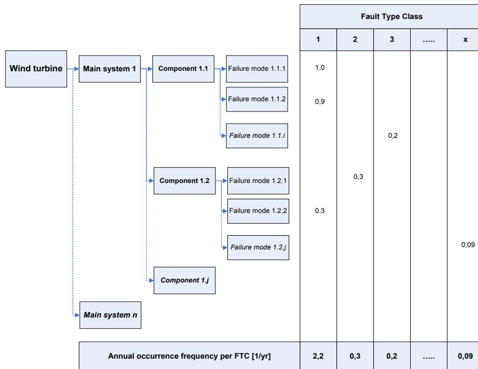
Figure A-4: *Process of grouping small and severe failures into manageable set of FTC's*
