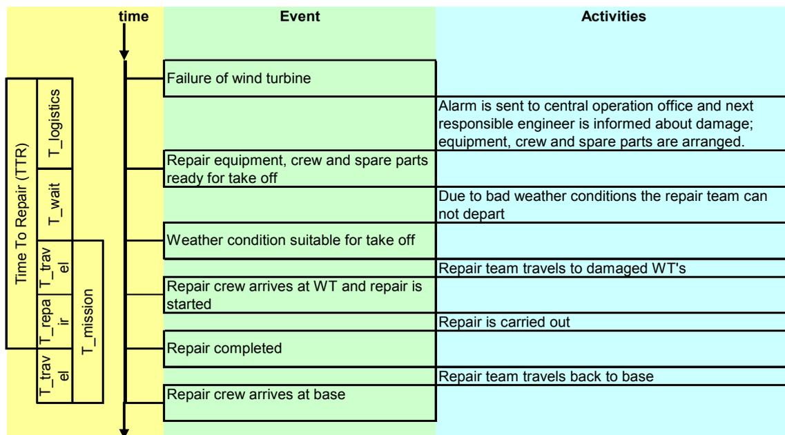
Figure A-2: *Repair process*
