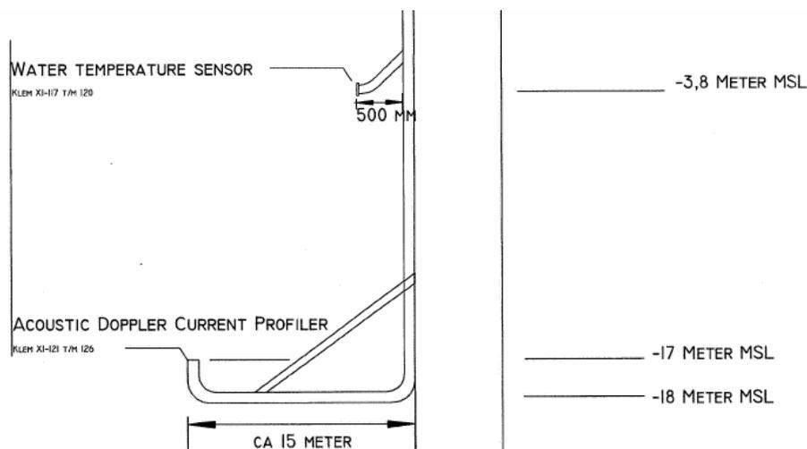
Figure 1.1 Position of the ADCP on the monopile of the meteorological mast.
