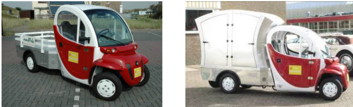
Figure 5: The HydroGEM FCV before(left) and after installation of the cooling unit (right)
