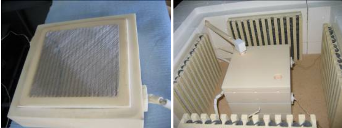
Figure 2.4 Ceramic cell housing used for the SOFC tests. The anode flange and current collecting mesh are shown on the left hand side, and the total set-up on the right hand side.
