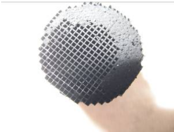
Figure 6.3 Carbon build-up on the inlet side of the catalyst structure when using nozzle concept B
