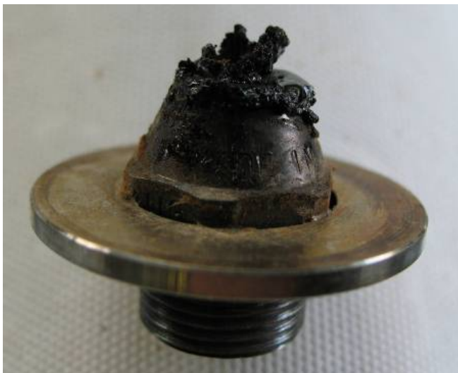
Figure 4.7 Carbon deposition on the nozzle
