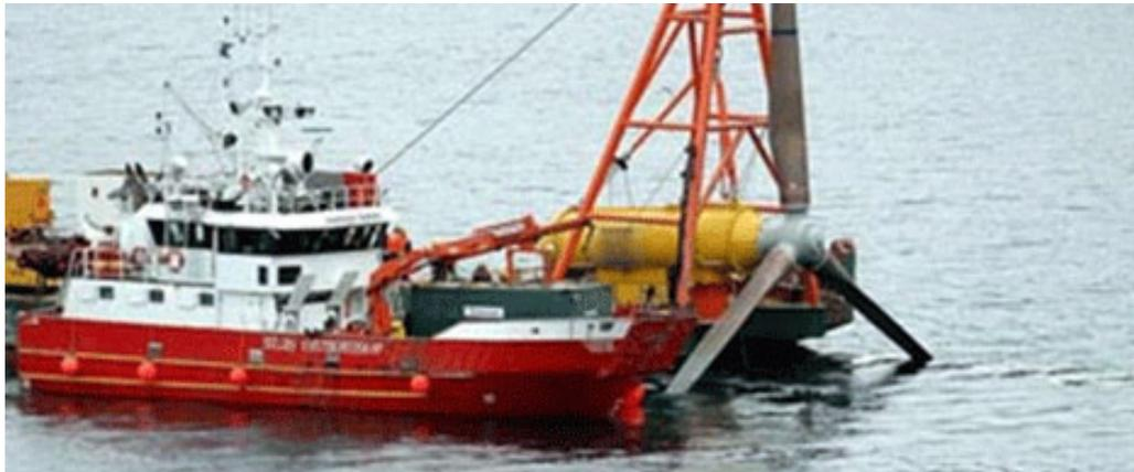
Figure 3.21 *Prototype tidal stream unit Hammerfest Strøm (parent company Statoil)*
