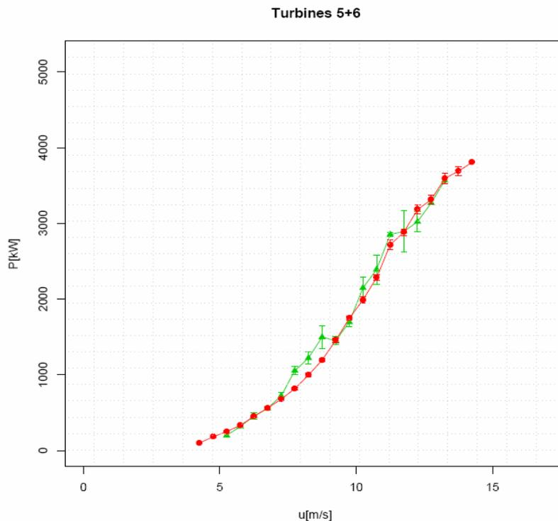
Fig. 5.6 Power performance characteristics of turbine 5 (left) and 6 (right) according to the IEC 61400-12-1 like power performance analysis for scenario 20xxx (green triangles) and scenario 00xxx (red bullets). Error bars denote the standard deviation. In [19] the method of analysis is described.
