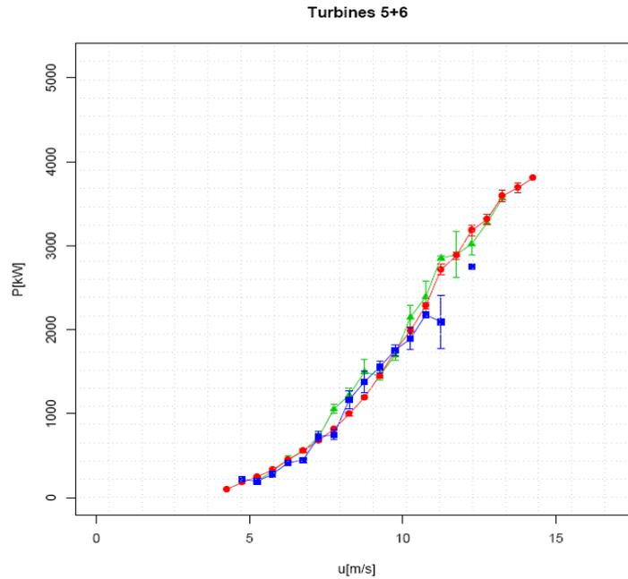
Fig. 5.7 Combined power performance characteristics of turbine 5 and 6 according to the IEC 61400-12-1 alike power performance analysis for scenario 40xxx (blue squares) 20xxx (green triangles) and scenario 00xxx (red bullets). Error bars denote the standard deviation. In [19] the method of analysis is described.
