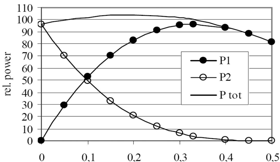
Fig. 5.1 The relative power production of two actuator disks in line with the wind. The downwind disc is fully in the wake of the upwind disc. The combination reaches maximum output (104.1%) at axial inductions of  $1/5$  for the upwind disk and  $1/3$  (Betz limit) for the downwind disc respectively.
