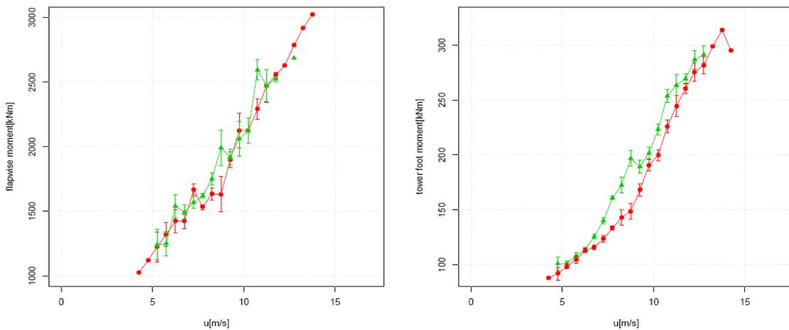
Fig. 5.9 Mean blade root flapwise moment of turbine 6 (left graph) and tower foot moment of turbine 6 (right graph) for scenario 20xxx (green triangles) and scenario 00xxx (red bullets). Error bars denote the standard error. In [19] the method of analysis is described.
