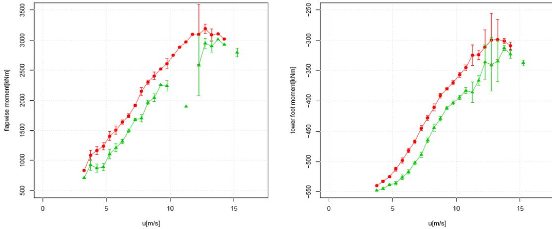
Fig. 5.8 Mean blade root flapwise moment of turbine 6 (left graph) and tower foot moment of turbine 6 (right graph) for “Heat and Flux” pitch (green triangles) and standard pitch (red bullets). Error bars denote the standard error. In [19] the method of analysis is described.
