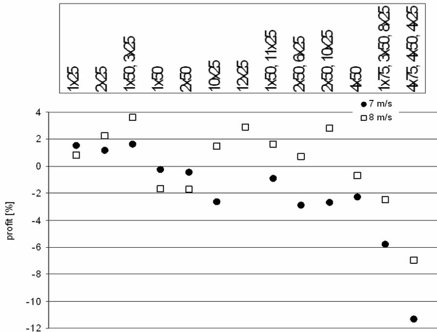
Fig. 5.4 Difference in total power produced by a row of 10 “Heat and Flux” model turbines compared with a row of 10 “conventional” turbines reported in [16]. The relative difference  $(P_{H\&F}-P_{conv})/P_{conv} \times 100\%$  is given for 7 and 8m/s tunnel speed and different combinations of pitch settings.
