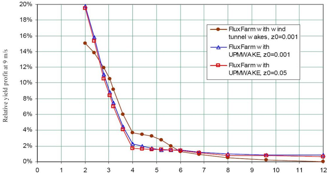
Fig. 5.2 Maximum relative power gain for “Heat and Flux” operation in a row of five EWTW type turbines in line with the wind direction as function of the turbine spacing in rotor diameters for a wind speed of  $9\text{ m/s}$ . The results are calculated [6] with FluxFarm and single wake maps derived from calculations (“UPMWAKE”) and wind tunnel measurements (“tunnel wakes”).
