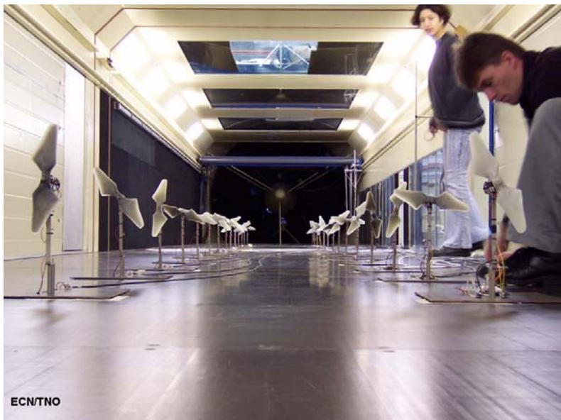
Fig. 3.1 *Installation of two rows of 14 turbines in the boundary layer wind tunnel of TNO: one row of models with “Heat and Flux” control and one row of models with conventional blade angles of  $0^\circ$ . The picture is taken in the direction of the flow.*
