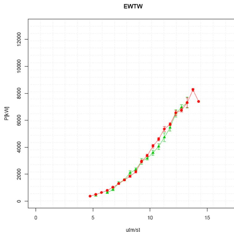
Fig. 5.5 Power performance characteristics of the EWTW according to the IEC 61400-12-1 alike power performance analysis for scenario 22220 (green triangles) and scenario 00000 (red bullets). Error bars denote the standard deviation. In [19] the method of analysis is described.
