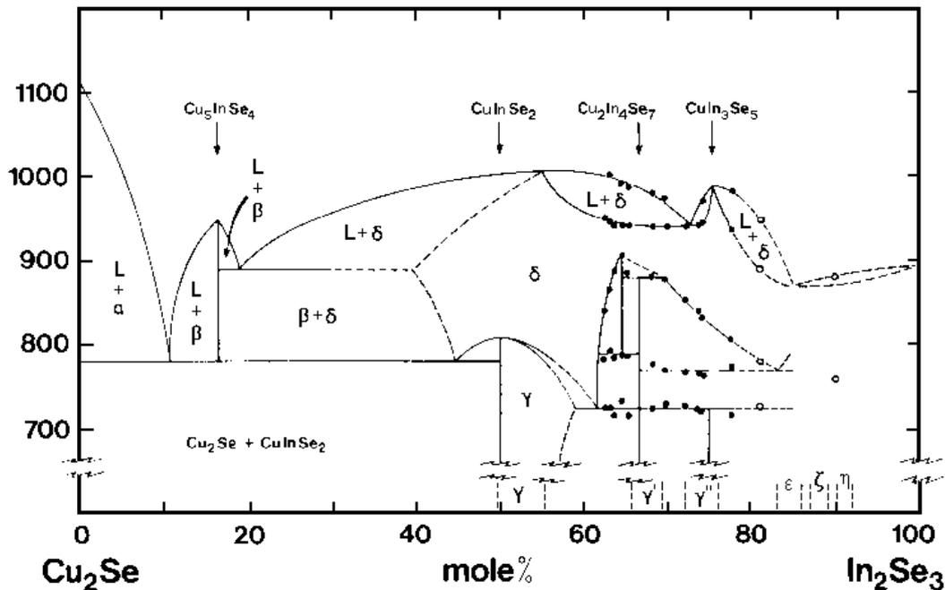
Figure 3 *Cu<sub>2</sub>Se – In<sub>2</sub>Se<sub>3</sub> pseudobinary phase diagram*
