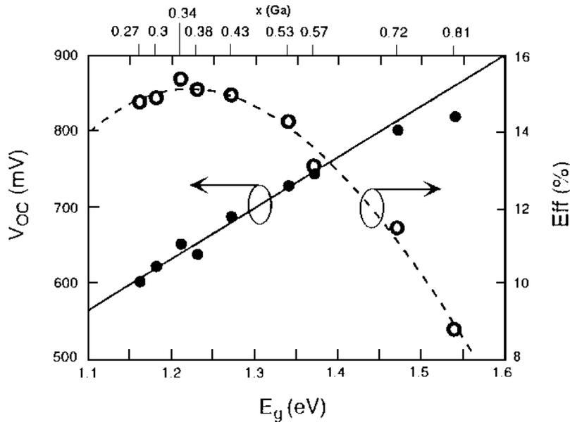
Figure 2 influence of Ga content on  $V_{oc}$  and efficiency
