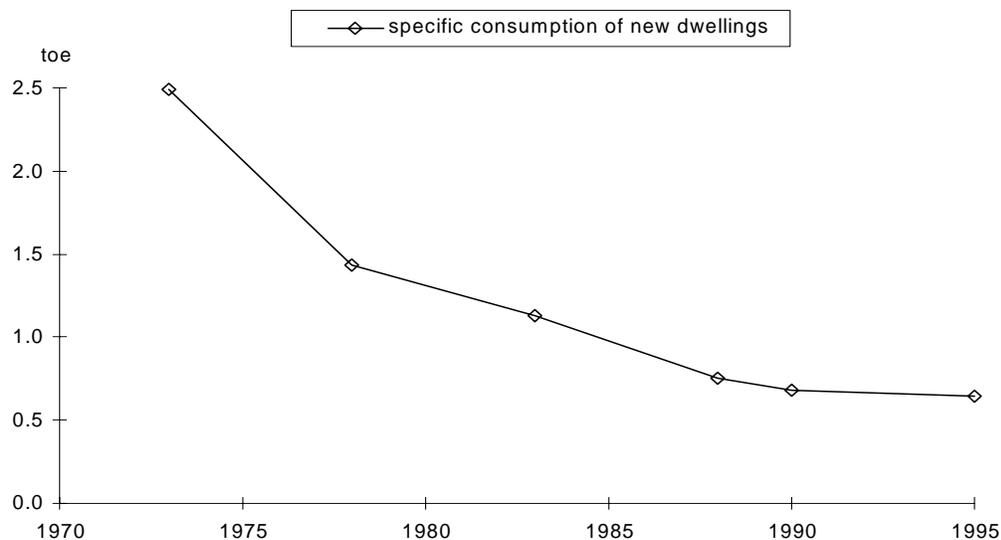
Figure 5.4 Specific consumption of new dwellings (incl. climatic corrections) [5,9,10]
