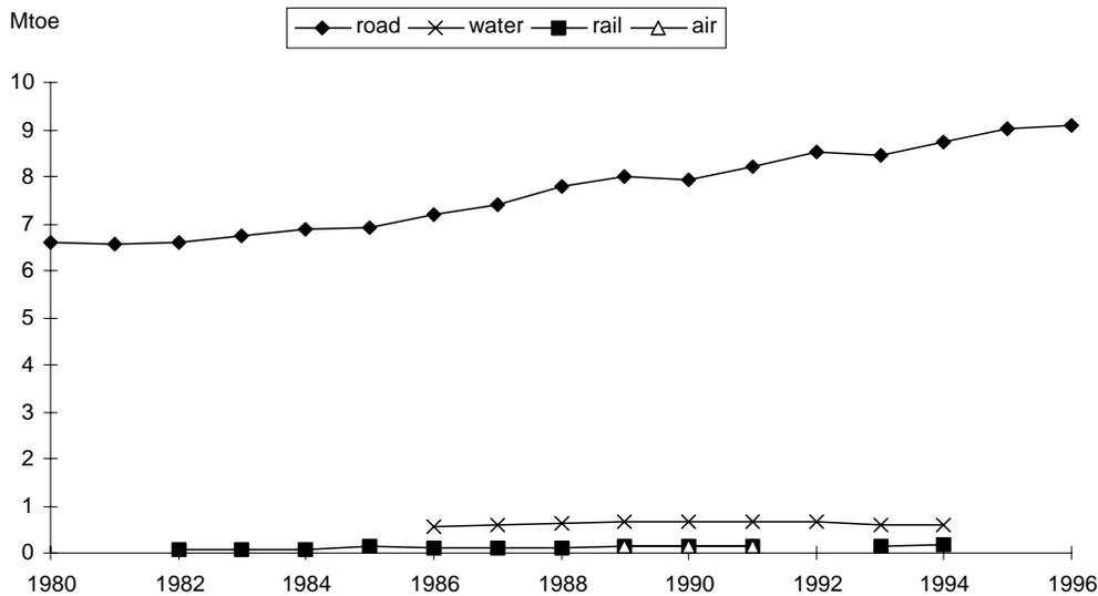
Figure 6.A *Transport energy consumption by mode*
