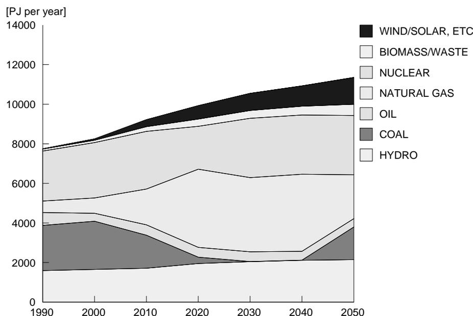
Figure 6.1 Power generation 1990-2050, 20 ECU/ton CO<sub>2</sub> case RP
