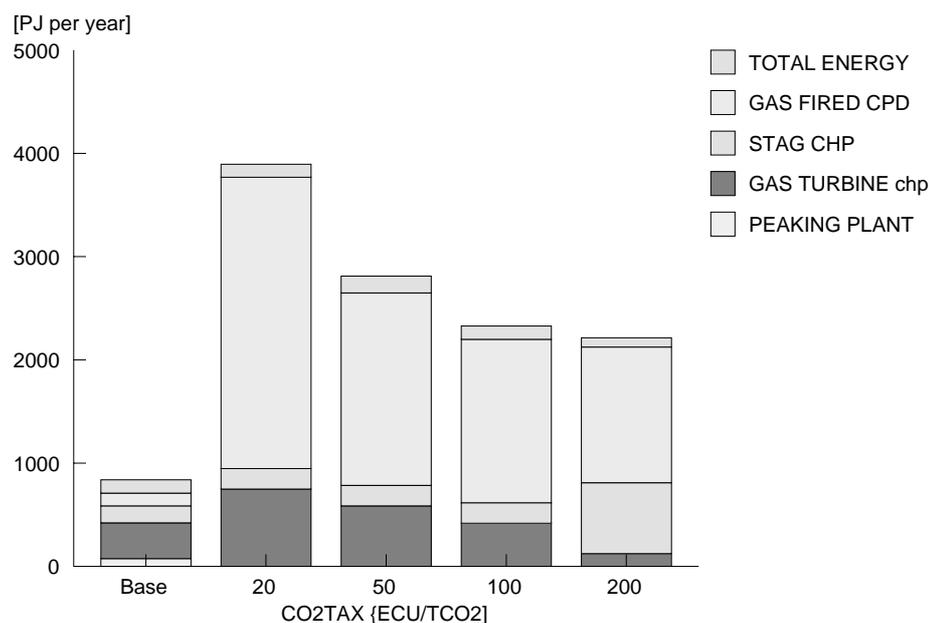
Figure 6.7 Gas fired power in 2040 as a function of carbon tax, RP
