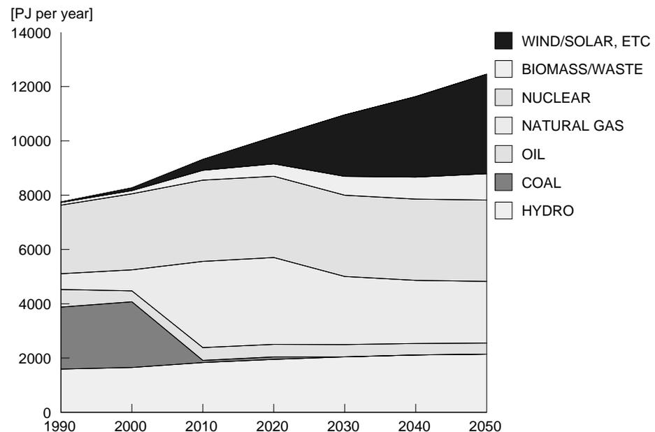
Figure 6.3 Power generation 1990-2050, 100 ECU/ton CO<sub>2</sub> case RP
