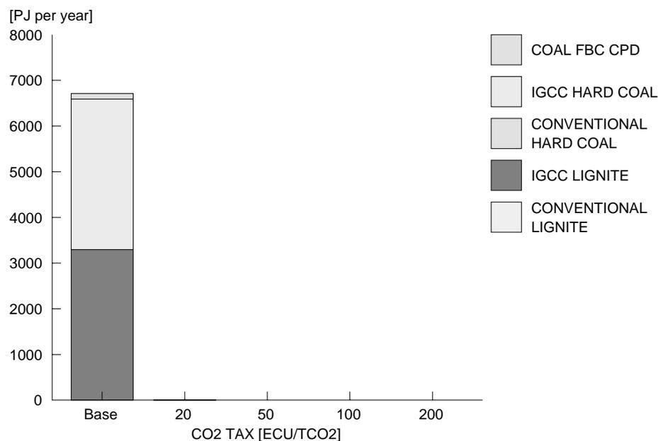
Figure 6.10 Coal fired power in 2020 as a function of carbon tax, RP
