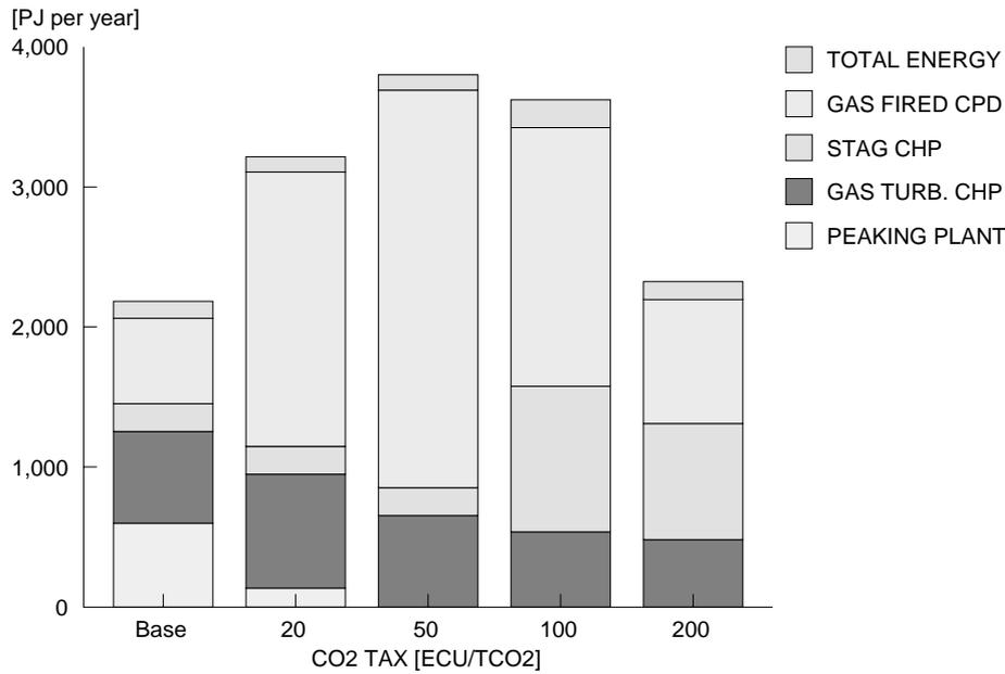
Figure 6.8 Gas fired power in 2040 as a function of carbon tax, MD
