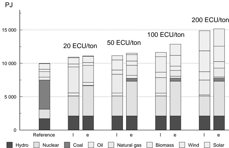
Figure 6.12 *Power generation mix in 2040 as a function of carbon tax, RP with or without relaxed attitude towards nuclear power, etc.*<sup>1</sup>
