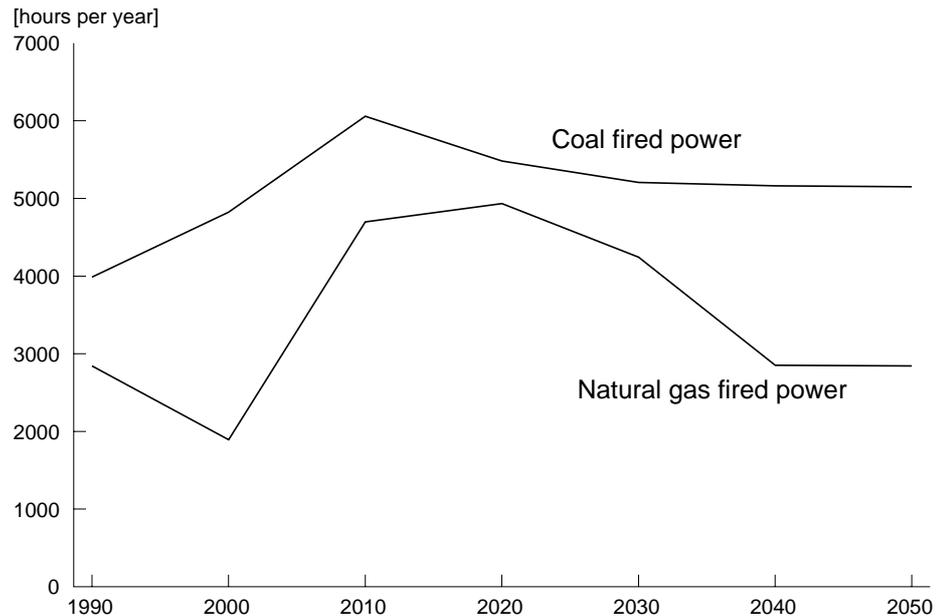
Figure 5.5 Full load hours of gas fired power and coal fired power, baseline projection scenario RP
