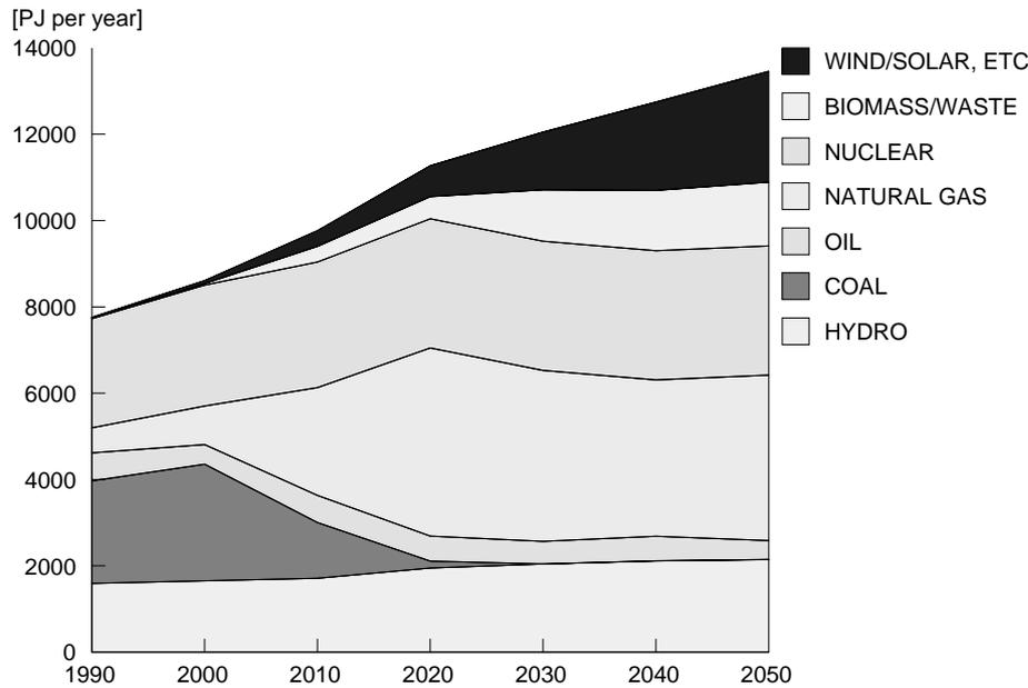
Figure 6.6 Power generation 1990-2050, 100 ECU/ton CO<sub>2</sub> case MD
