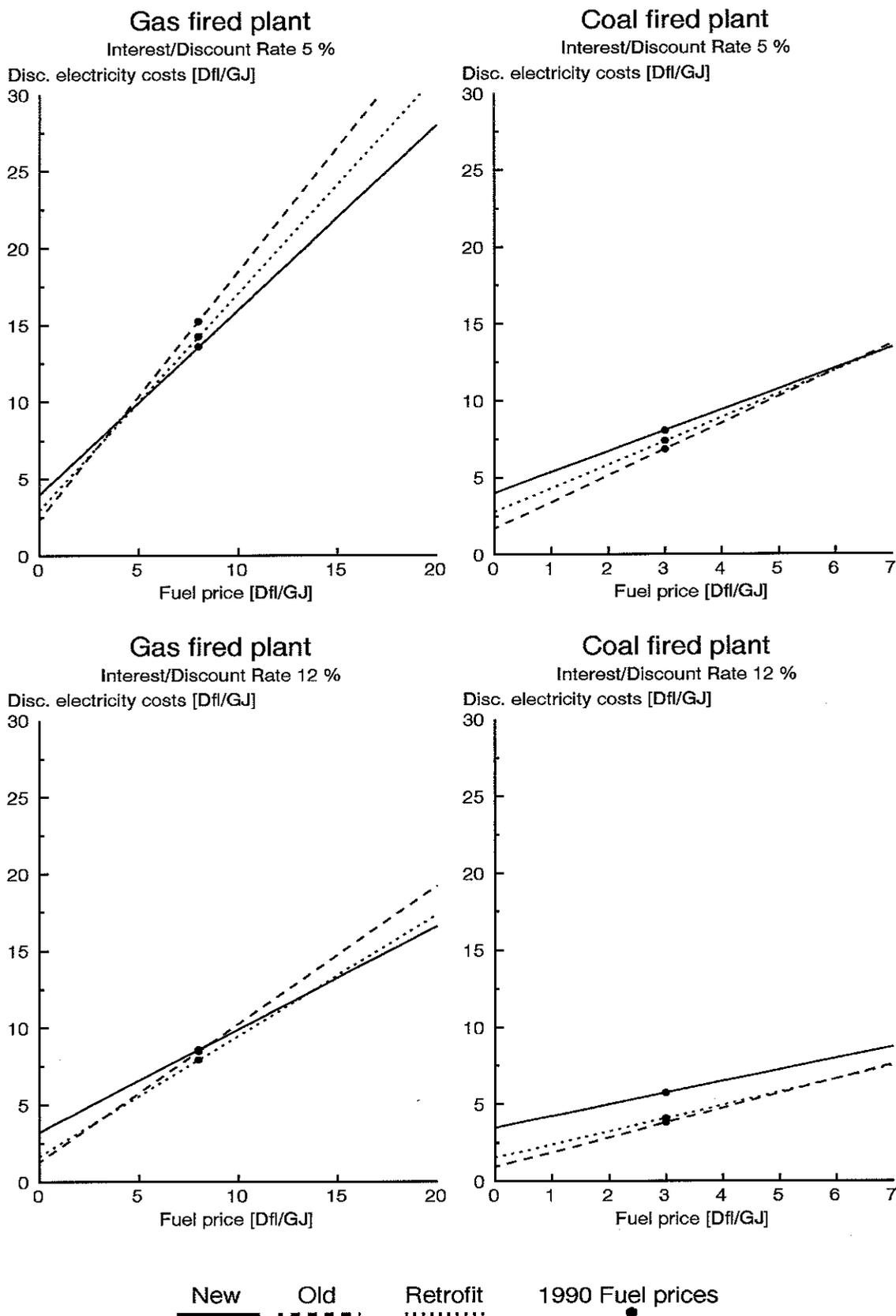
Figure 5.1 Discounted electricity production costs of old, new, and retrofitted gas fired and coal fired power stations as a function of the fuel price, using 5% and 12% discount rate
