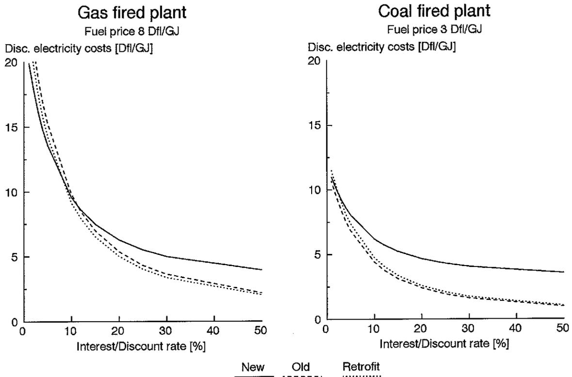
Figure 5.2 *Discounted electricity production costs of old, new, and retrofitted gas fired and coal fired power stations as a function of the interest and discount rate, using approximately current fuel prices*
