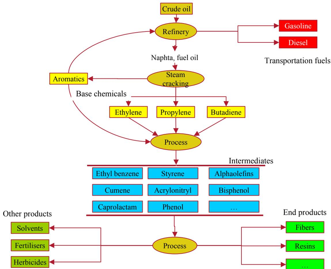
Figure 2.7 Simplified scheme of the material flows in the petrochemical megasite
