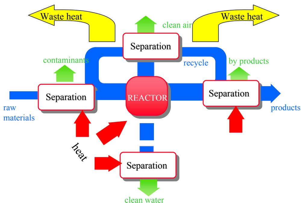
Figure 2.6 *Key energy aspects of the chemical process: reactions, separations and thermal integration*
