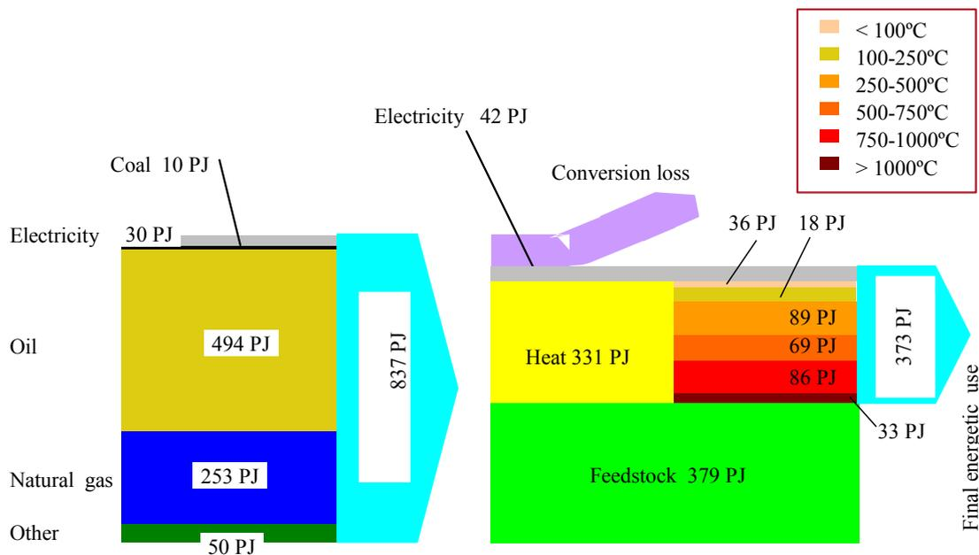
Figure 2.4 Energy balance for the Dutch chemical and refining industry in 2000 in PJ/year (Spoelstra, 2005)
