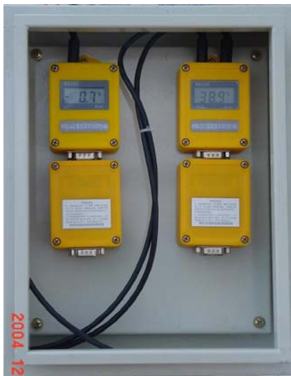
Figure 3.11 Data recording devices as installed in the project Greenhouses
