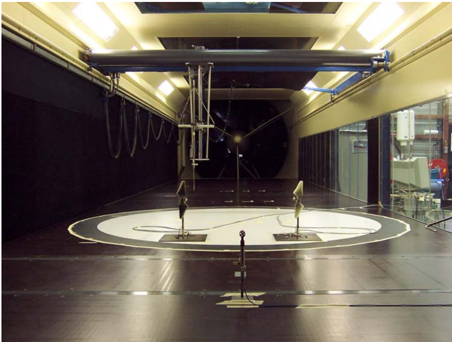
Figure 2.2 View of the measurement section of the tunnel with the traverse system. In the front center the Schiltknecht anemometer is placed on the floor. In the back of the tunnel the fan can be seen.
