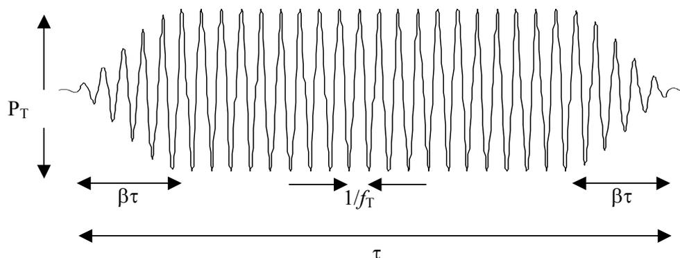
Figure 2.1 Basic pulse shape of the Sodar
