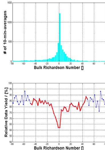
Figure 4.1. Upper panel: Distribution of Bulk Richardson number as observed from 2003-05-23 to 2003-07-23. Lower panel: Percentage of relative data yield of Sodar receptions for the same period, plotted versus the Bulk Richardson number.
