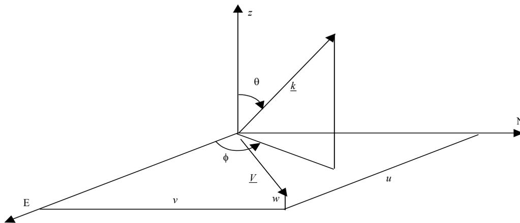
Figure 2.12 Orientation of the Sodar beams
