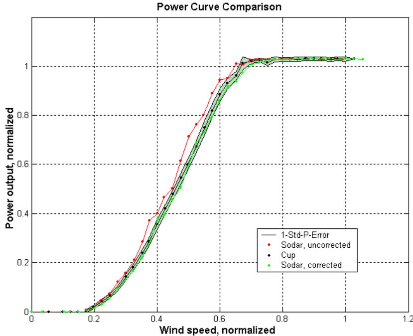
Figure 5.4 Power performance curves for the three prescribed approaches. Grey shaded tube represents the 1-std-error-bar for the PPC as recorded by the cup anemometer at the met mast.
