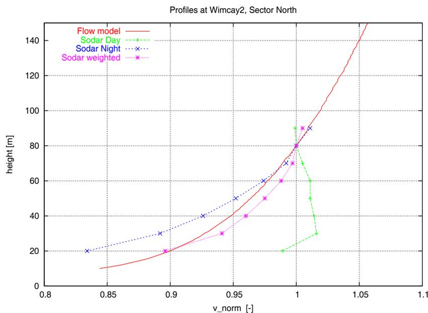
Figure 6.7. Normalized profile as computed with flow model and derived from the Sodar data.
