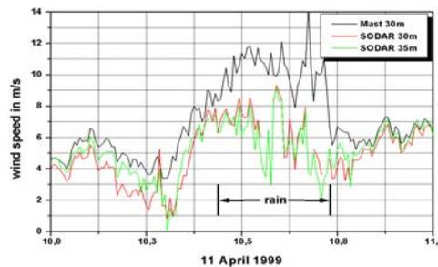
Figure 4.2. Sodar and met tower readings during dry and rain weather
