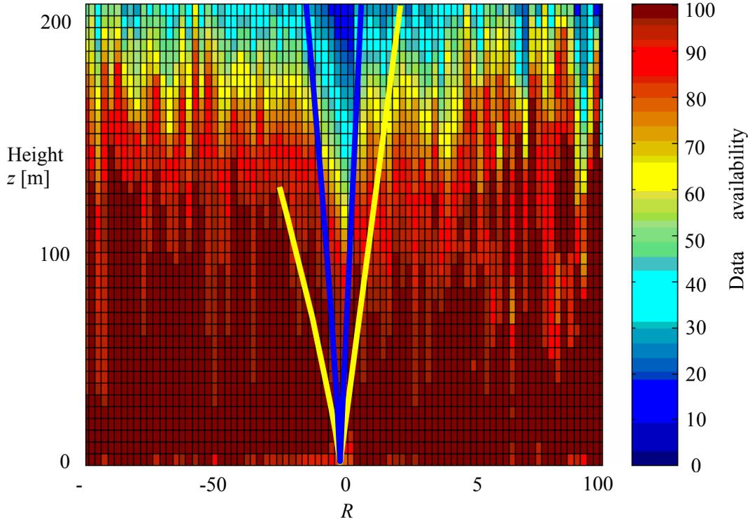
Figure 3.2 Percentage of relative data yield of Scintec Sodar receptions, plotted against height  $z$  of the Sodar range gates and against the Richardson number  $Ri$  based on meteorological mast measurements at 100 m. The solid yellow and blue lines are two contours of constant  $\frac{C_T^2}{z^2}$  based on the theory developed in WP3.
