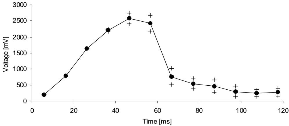
Figure 2.11 Transducer signal due to ringing where time = 0 ms is the time when the pulse has finished being sent.
