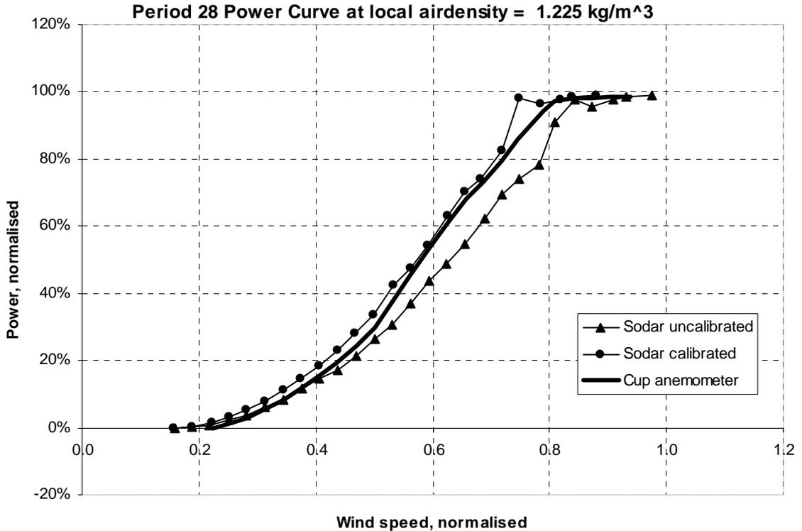
Figure 5.3 Power curves for the calibration period.
