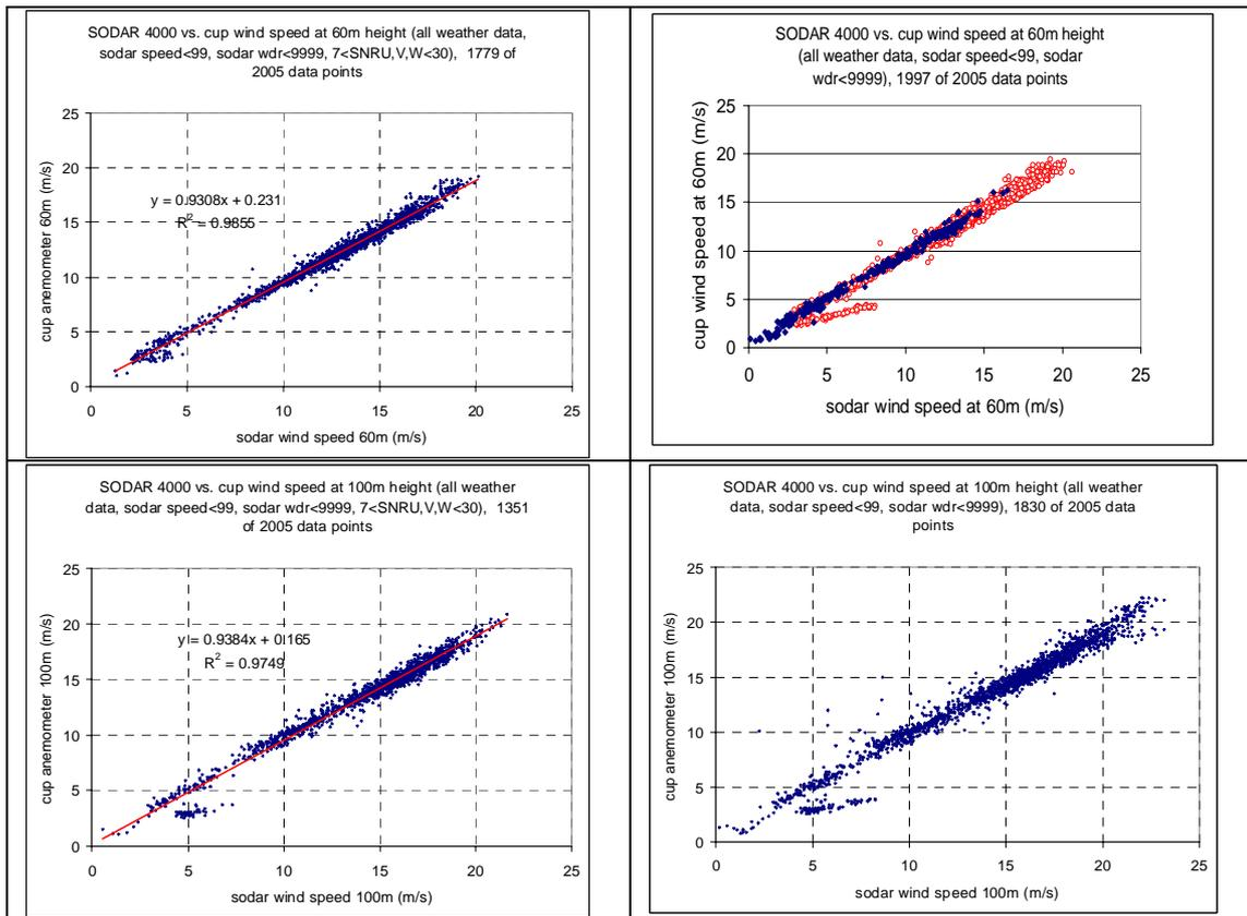
Figure 4.6 Filtered and non-filtered Sodar wind speed data at 60m and 100m height. In the right upper figure results are shown as rain (red circles) and dry (blue solid) weather data.
