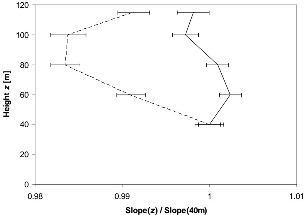
Figure 3.5 Variation in slope  $m'$  with height. Metek (dashed line), AeroVironment (solid line).
