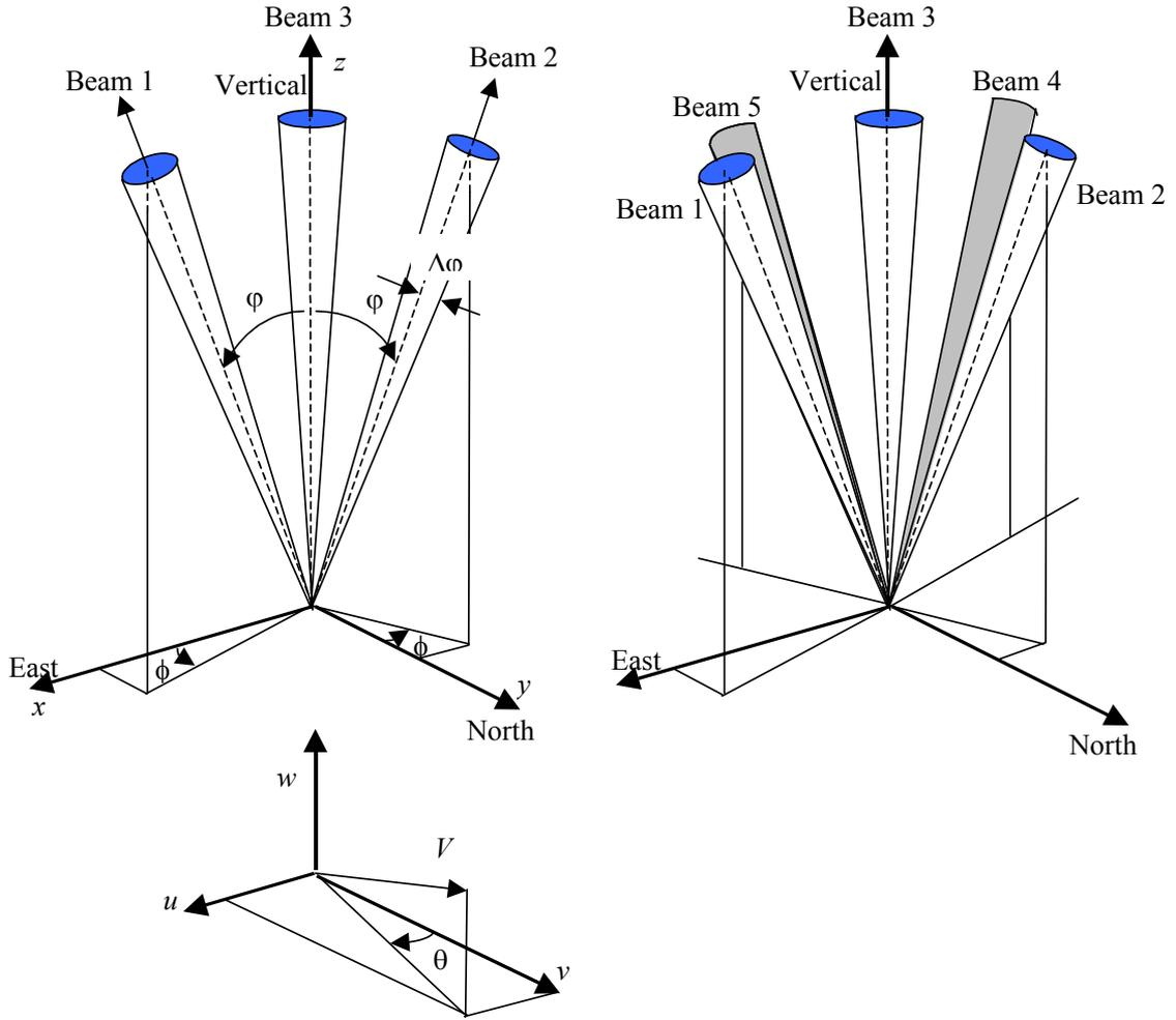
Figure 3.1 Typical beam geometries for a 3-beam and a 5-beam system, showing the relationship to wind components.
