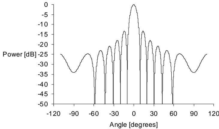
Figure 2.10 Antenna beam pattern with baffle.
