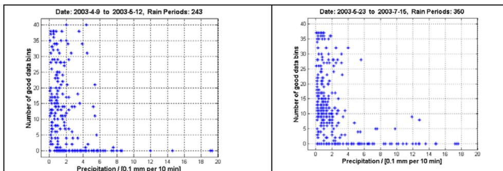
Figure 4.3. Dependency of the number of valid data returns on the precipitation rate
