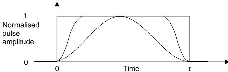
Figure 2.6. Time series of square window compared to Hanning shaped pulse with different ramp times.
