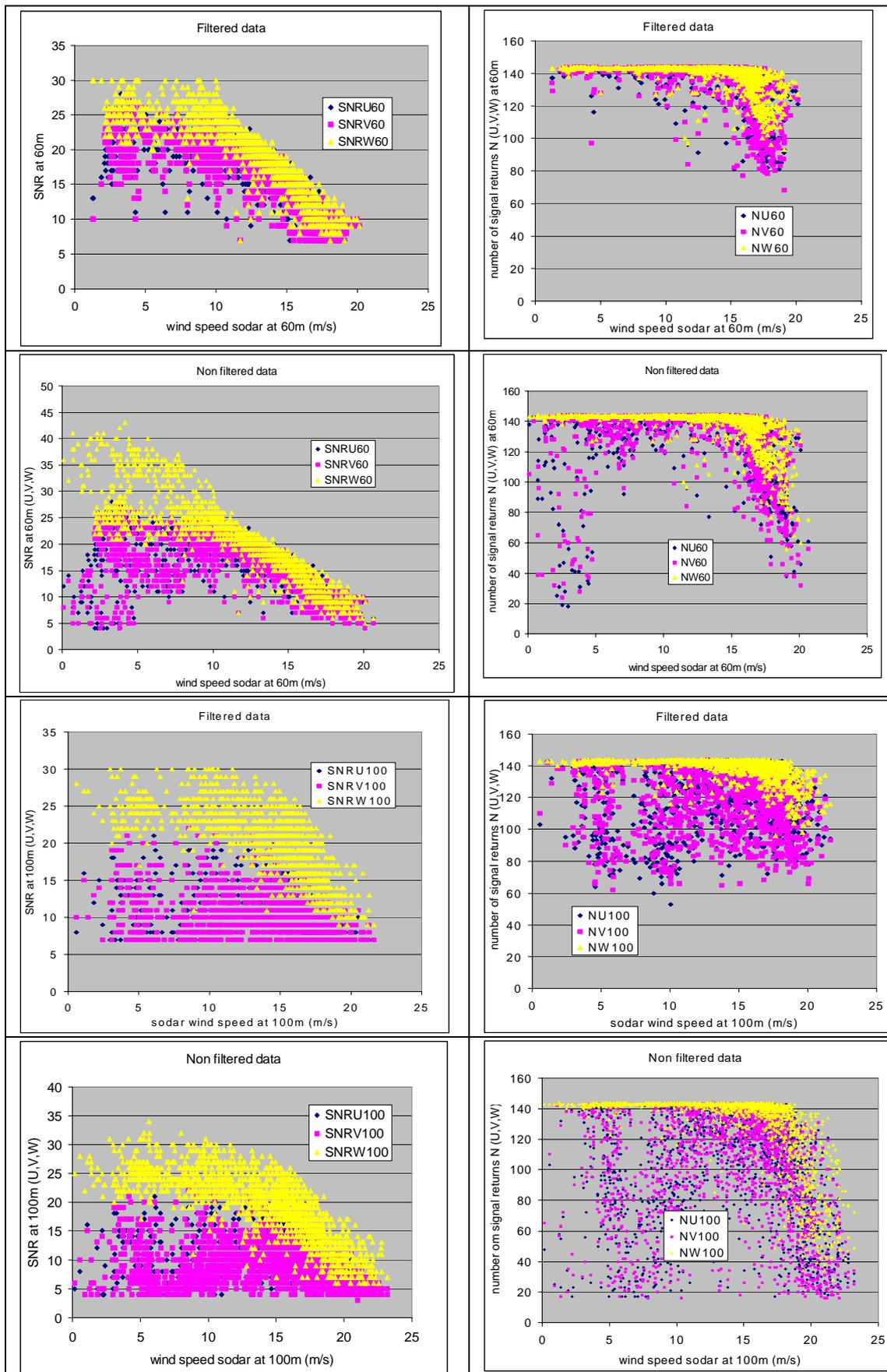
Figure 4.7. The SNR and the number of signal returns (filtered and non-filtered data) at 60m and 100m height.
