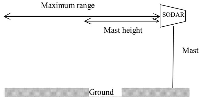
Figure 6.8. Scetch of a nacelle or mast based Sodar.
