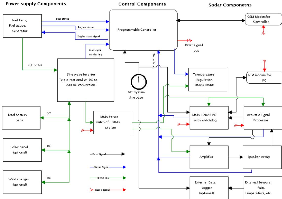
Figure 6.2. Scheme for a Sodar with autonomous power supply.
