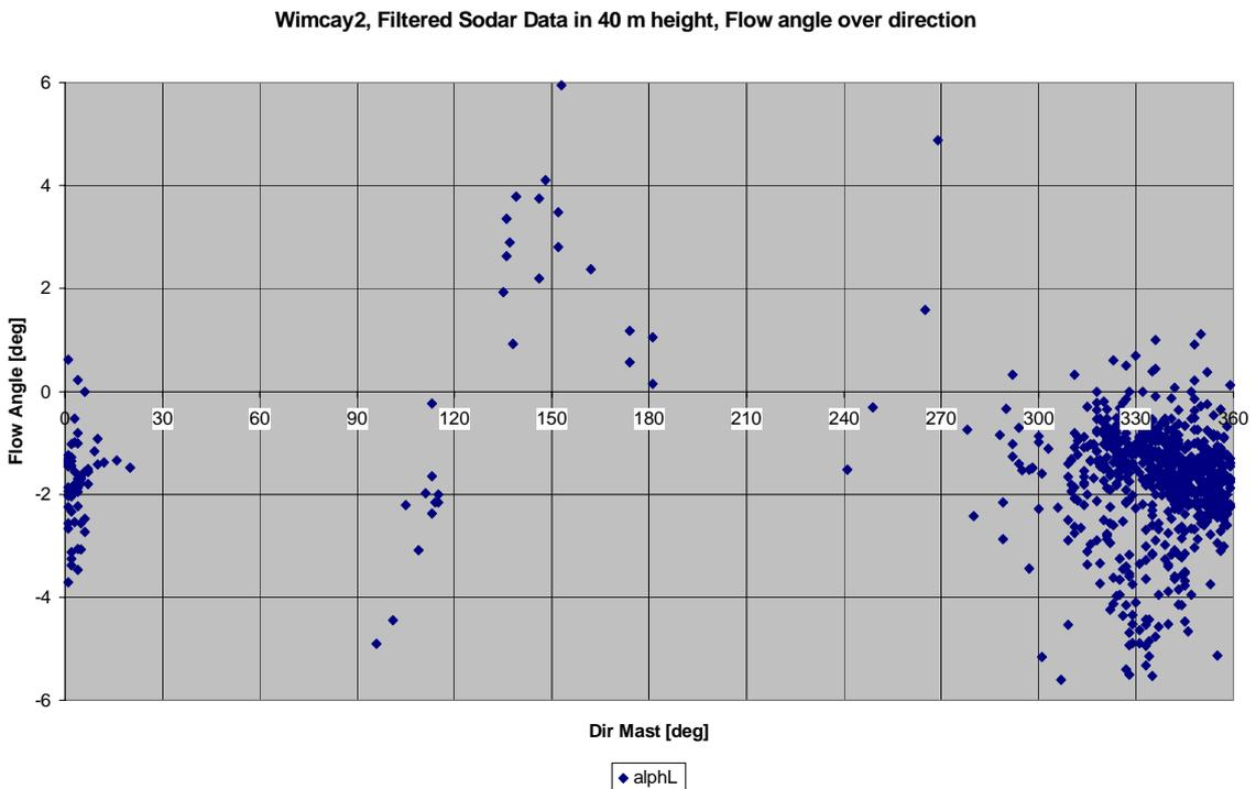
Figure 6.5. Example of flow inclination measurement with the Sodar.
