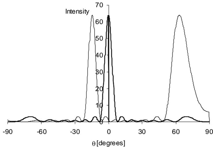
Figure 2.8 Antenna beam pattern for a line array consisting of 8 speakers with a speaker spacing of  $0.95\lambda$  and at a transmit frequency of 4500 Hz. The vertical beam corresponds to the thick line, the tilted beam to the thin line.
