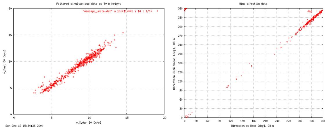
Figure 6.3 Example of a filtered data set for 80 meters height in comparison with the met mast data.
