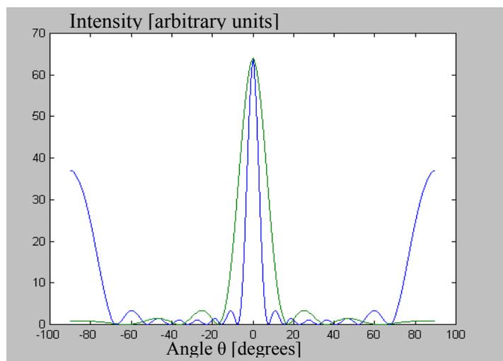
Figure 2.9 Antenna beam pattern (for details see Fig. 6) at two different transmit frequencies: Blue – 4500 Hz, green – 2000 Hz.
