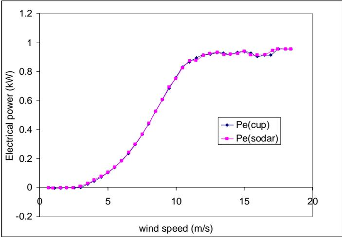
Figure 5.2 The power curve as a function of the wind speeds measured by the cup and the Sodar.
