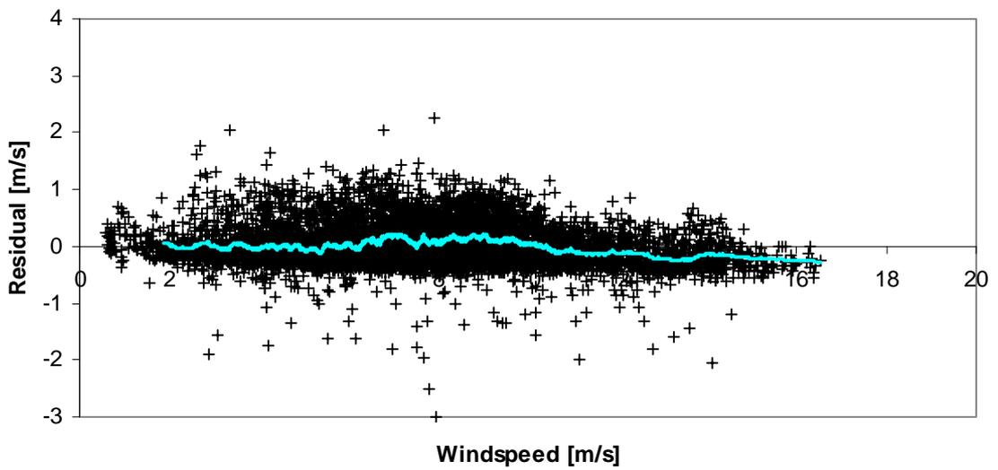
Figure 3.4 Upper plot: Residual plots for AV4000 Sodar and cup at 60m. Lower plot: Residuals in a linear fit of 80 m cup wind speed to 60 m cup wind speed. Superimposed line: running average of 100 points.
