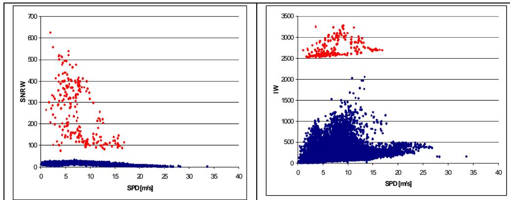
Figure 4.5 The signal to noise ratio and the signal intensity vs. the wind speed
