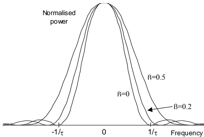
Figure 2.7. Frequency spectra of a square pulse compared to Hanning shaped pulse with different ramp times.
