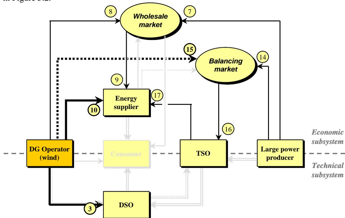
Figure 5.2 Power storage device implemented by the DG operator
