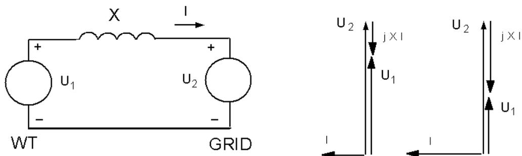
Figure 3.5 *Effect of the reactive power on voltage  $U_1$*
