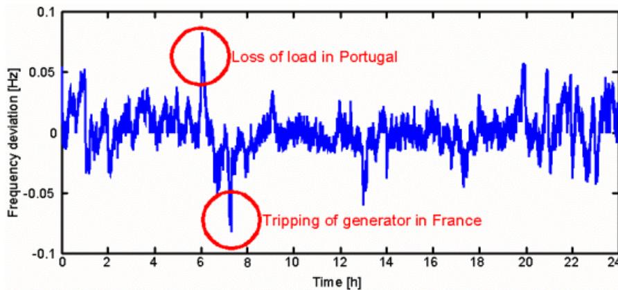
Figure 3.3 *Two events in the European Electrical Power System on January 10, 2001 leading to frequency excursions (Slootweg)*
