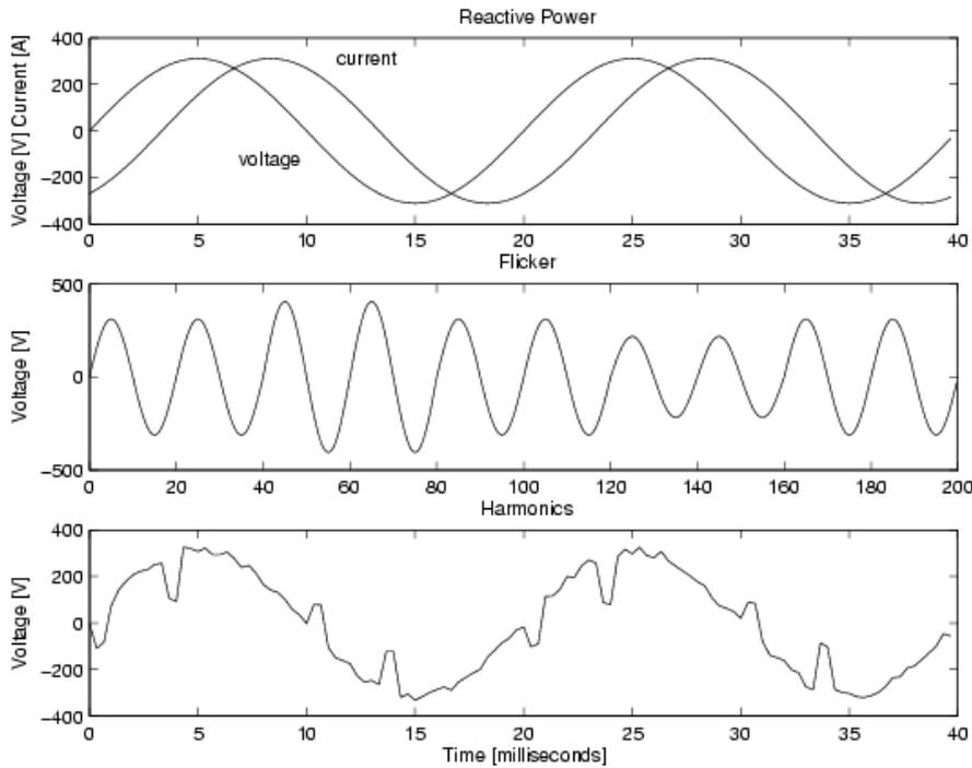
Figure 3.4 *Illustration of the different aspects of power quality*
