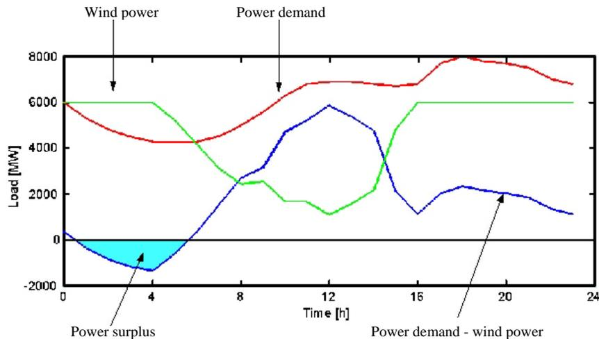
Figure 3.6 Example of a power surplus in a grid control area (Slootweg)
