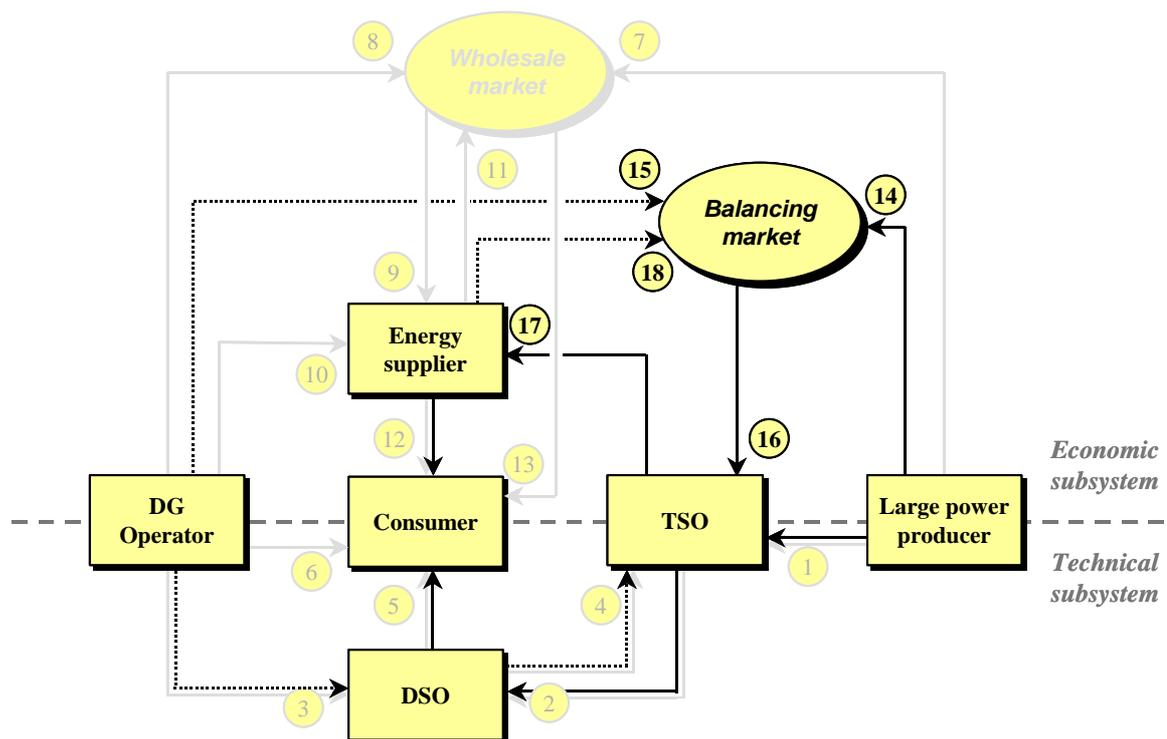
Figure 2.2 Overview of transactions within the electricity market, including the balancing market
