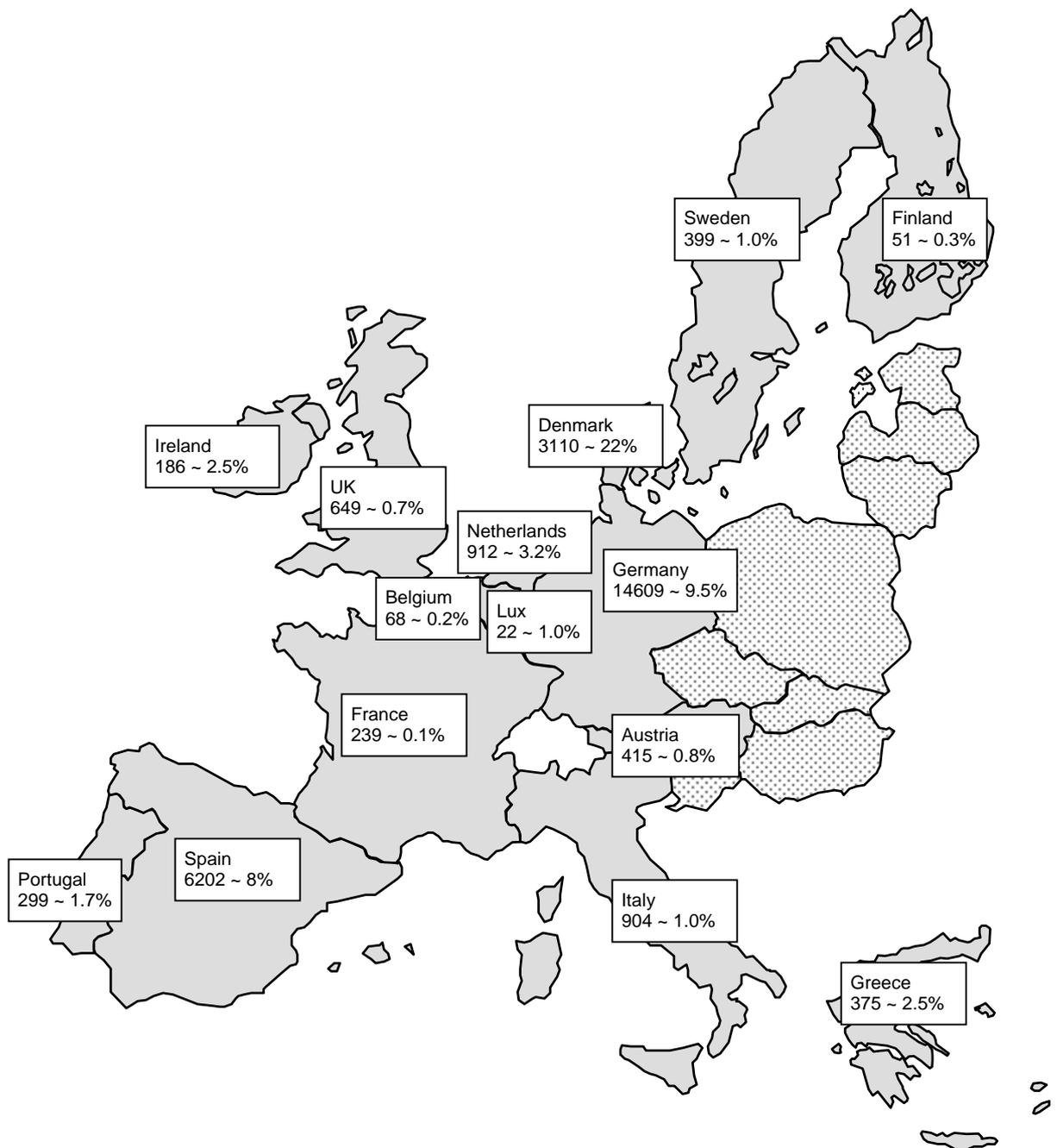
Figure 3.2 *Wind power installed in Europe by the end of 2003 (in MW and as a fraction of total generating capacity per country)*
