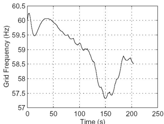
*Frequency dip of the Costa Rica grid in isolated operation resulting from a shutdown of 198 MW wind power in three minutes (Pierik and Montero)*
