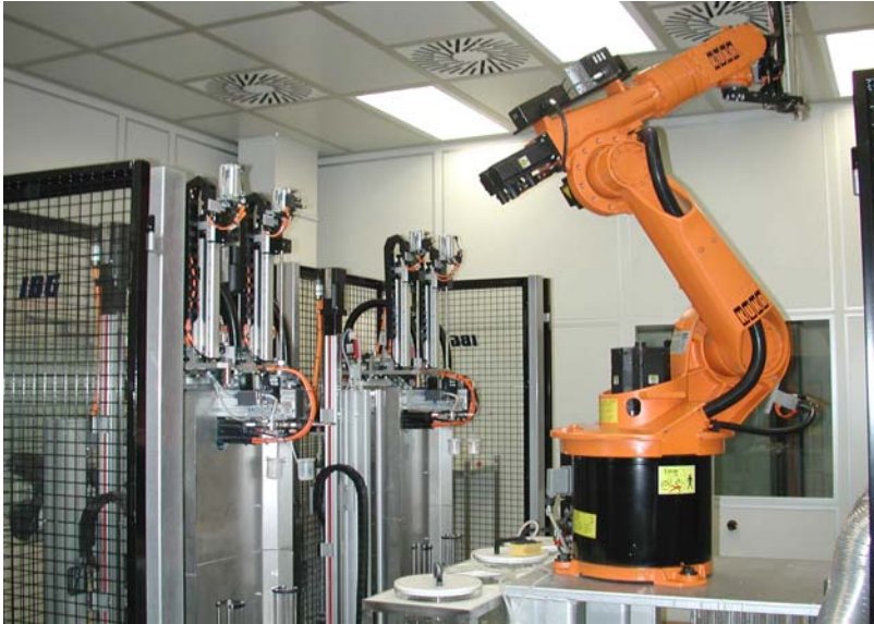
Figure 2.32 Coating robot in clean room and coating stations
