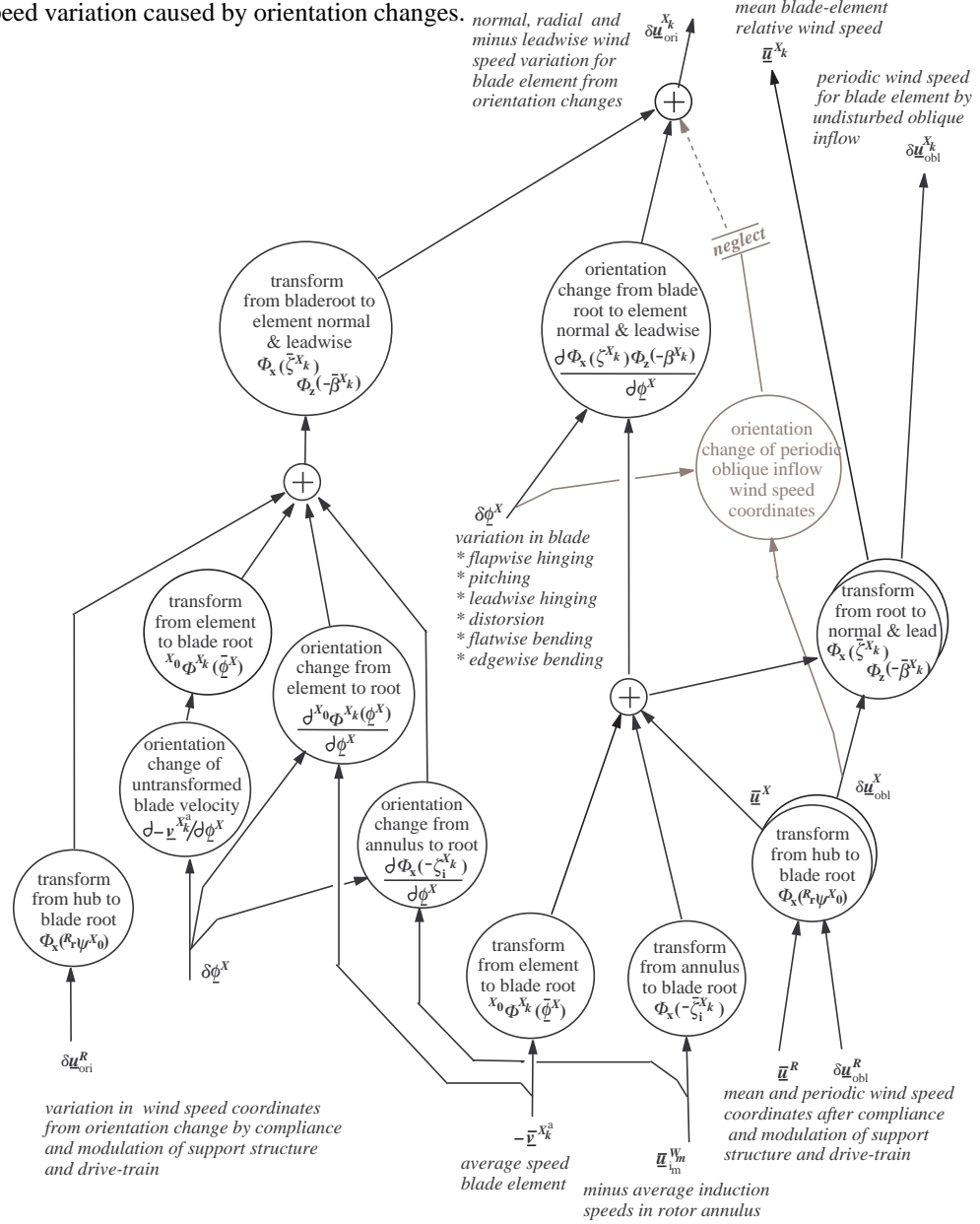
Figure B.3 Wind speed coordinates on blade element from mean longitudinal wind speed, mean induction speed and mean blade speed
