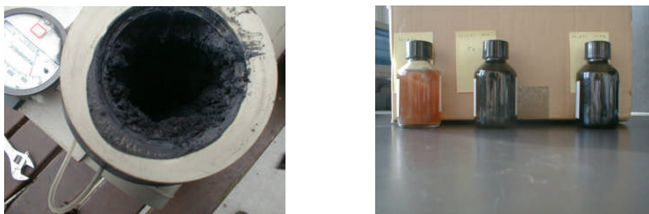
Figure 1.1 Tar related problems of fouling (left) and wastewater production (right) in a biomass gasification process.
