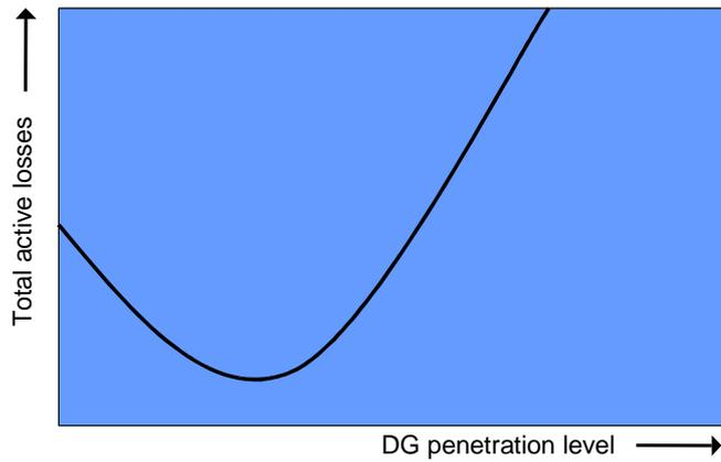
Figure 4.1 *Variation of distribution losses due to DG penetration*
