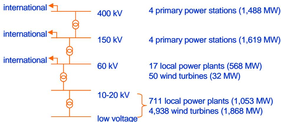
Figure 2.2 Production capacity at each voltage level in the Western part of Denmark (Eltra)
