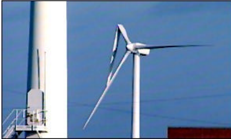
Fig. 1.1: Blade failure of an offshore wind turbine in Blyth Harbour (UK) due to a lightning strike [11,12]
