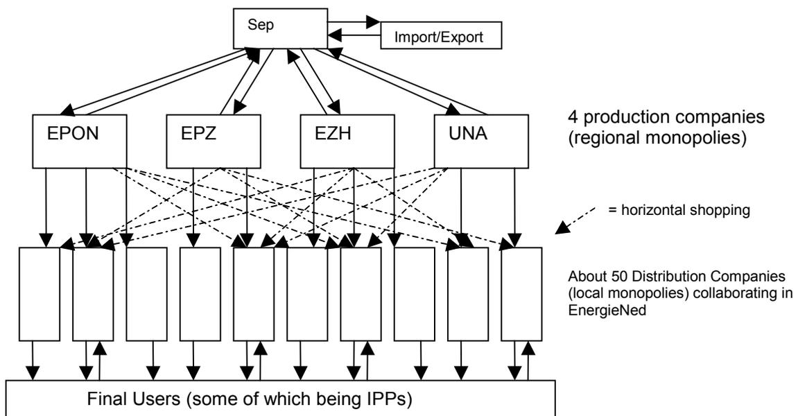
Figure 2.2 *Structure of the Dutch Electricity sector in the early 1990s, based on the Electricity Law of 1989*
