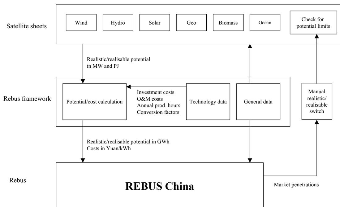
Figure 4.12 *REBUS-China modelstructure*
