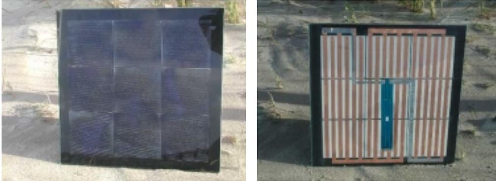
Figure 12: Rear- and front side of an EWT minimodule. The solar cells are manufactured without busbar. The interconnection of the fingers is made with conductive adhesive to the copper strips. The white isolation layer is a screen printable ceramic.
