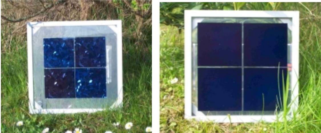
*Figure 2: Mini modules made of four EWT cells each. Multi-crystalline cells on the left, Cz-Si on the right. The Cz-module was measured at ECN and had an efficiency of 14.0 % (active module area).*
