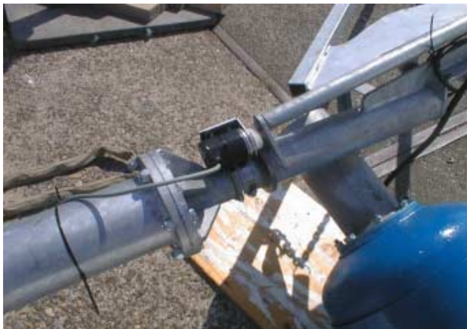
Figure A.2 Yaw measurement equipment
