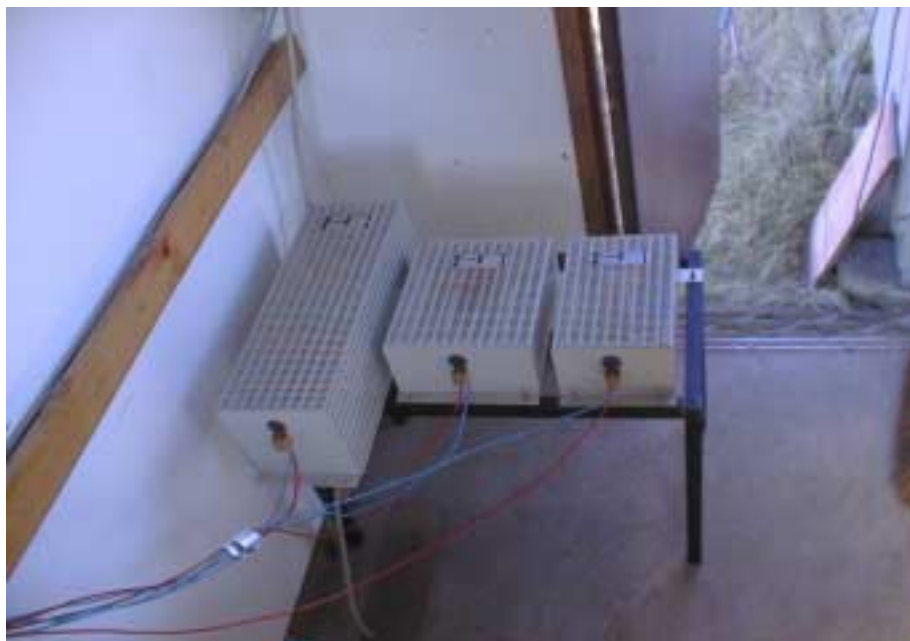
Figure A.6 Binary resistor bank acting as simulated load
