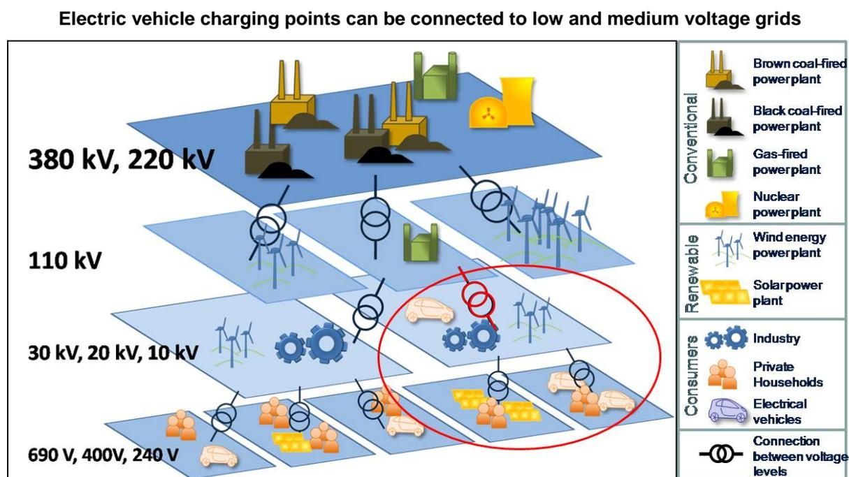
Figure 17 Composition of the electrical grid from the power generation to the point of consumption [IFHT, RWTH Aachen]
