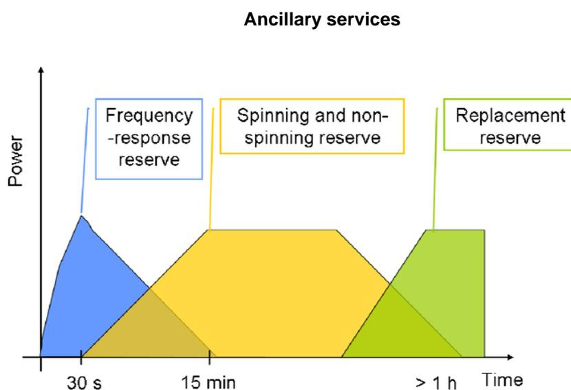
Figure 20 Representation of the different kinds of reserve power and the time intervals they are used in after
