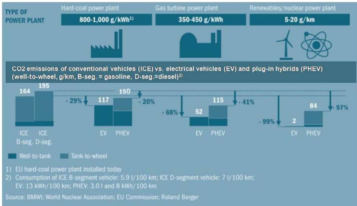
Figure 7 Comparison of CO<sub>2</sub> emissions from electric vehicles (EV) and plug-in hybrid vehicles (PHEV) with those of conventional, internal combustion engine vehicles (ICE) [RB Powertrain]
