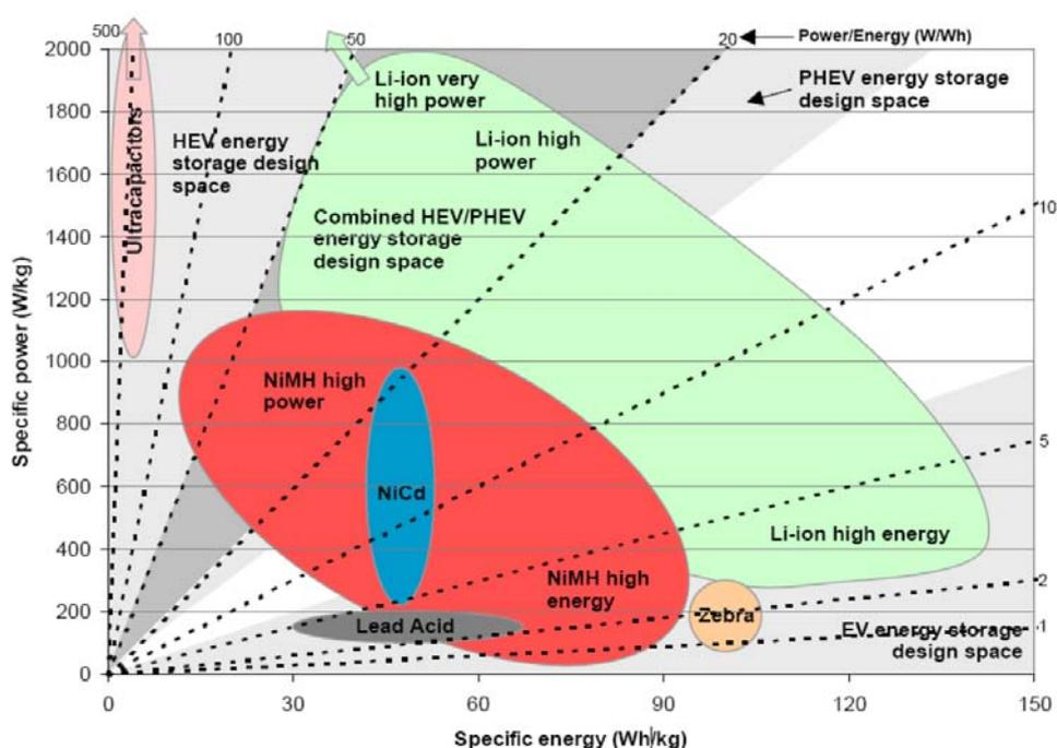
Figure 6 Comparison of specific energy and power for a range of battery types (Source: [BERR, 2008], based on data from Ricardo)
