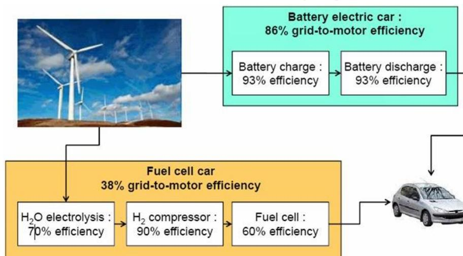
Figure 15 Comparison of the energy efficiency for bringing renewable electricity to the electric motor of a fuel cell and battery-electric car [Enerdata 2009]
