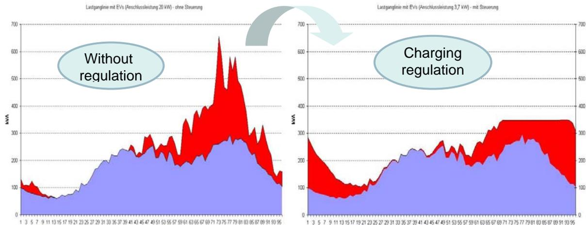
Figure 18 Example for a charging regulation, penetration rate per household 80% [IFHT, RWTH Aachen]
